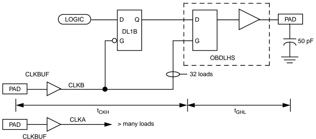
A3265DX-2  $T_{\text{CO}} = t_{\text{CKH}} + t_{\text{GHL}} = 5.1 \text{ ns} + 4.6 \text{ ns} = 9.7 \text{ ns}$
