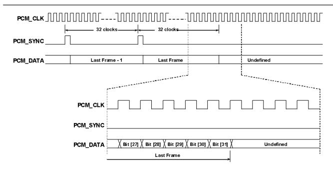
Note: Bit [31] is the last bit of the packet. No PCM\_SYNC pulses following the PCM\_SYNC pulse prior to the last frame.
