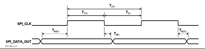
Figure 2-2 • SPI Receive Timing, ZL70250 to External Microcontroller
