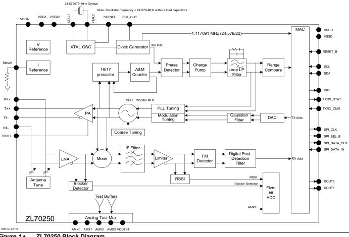
Figure 1 • ZL70250 Block Diagram
