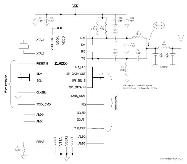
*Figure 5-1* • **50**-Ω Single-Ended Implementation Schematic
