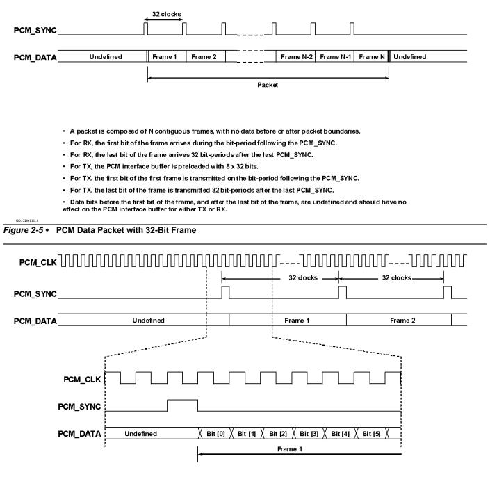
Note: Bit [0] is the first bit of the packet. No PCM\_SYNC pulses occur prior to the pulse immediately preceding bit [0].
