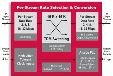
The ZL™ 50050/51/52/53/57/58/60/61/62/63/64 are Zarlink's series of feature-rich TDM switching ICs. The series includes 8 K, 12 K and 16 K channel devices capable of up to 32 Mbps data rates on all streams. With exceptional jitter tolerance, as well as the industry's widest range of per-stream and per-channel programmable features, Zarlink's new switching ICs are ideal for a variety of high-capacity carrier-class equipment.
