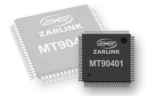
The MT90401 is a digital phase locked loop (DPLL) that synchronizes SONET (Synchronous Optical Network) and SDH (synchronous Digital Hierarchy) network equipment. The device uses an integrated approach to ease system design and reduce board space compared to traditional clock design or clock modules.
