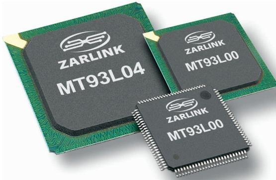
The MT93L00 and MT93L04 multi-channel voice echo cancellers provide advanced digital echo cancellation in multi-service ATM, SONET/SDH and wireless networks. The devices use a patented algorithm to provide unprecedented performance in a highly integrated solution that reduces cost and power consumption compared to alternative approaches.
