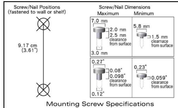
2. Align the PD-9501G mounting slots to capture the surface screws
