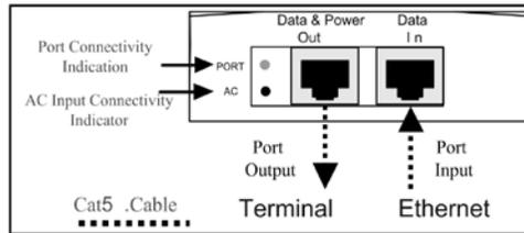
Figure 1: connecting the PoE Midspan
