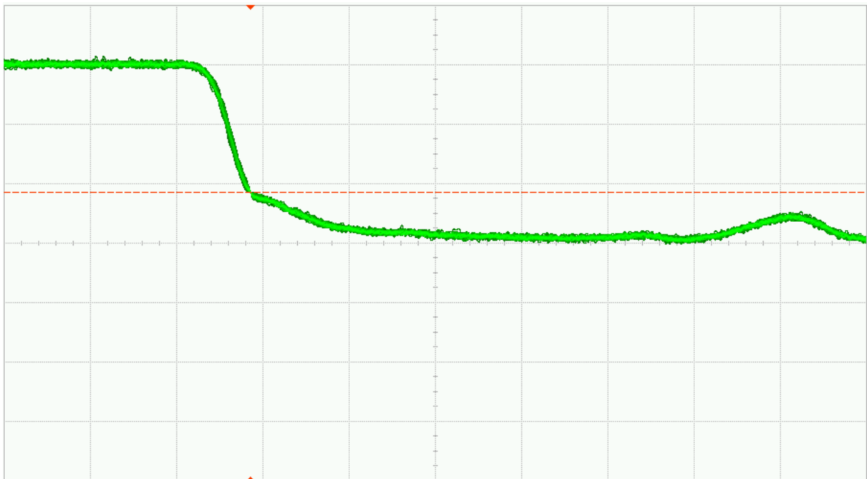
Fig. 34 (b). DUT 07287 post-annealing falling edge, abscissa scale is 1V/div and ordinate scale is 2ns/div
