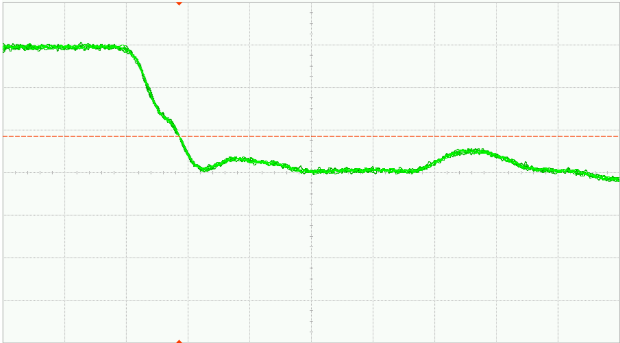
Fig. 35 (a). DUT 01850 pre-irradiation falling edge, abscissa scale is 1V/div and ordinate scale is 2ns/div
