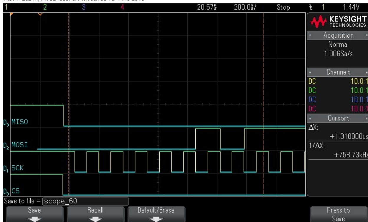
Figure 9-119. Read Command. Command = 0x5. Note CS signal
