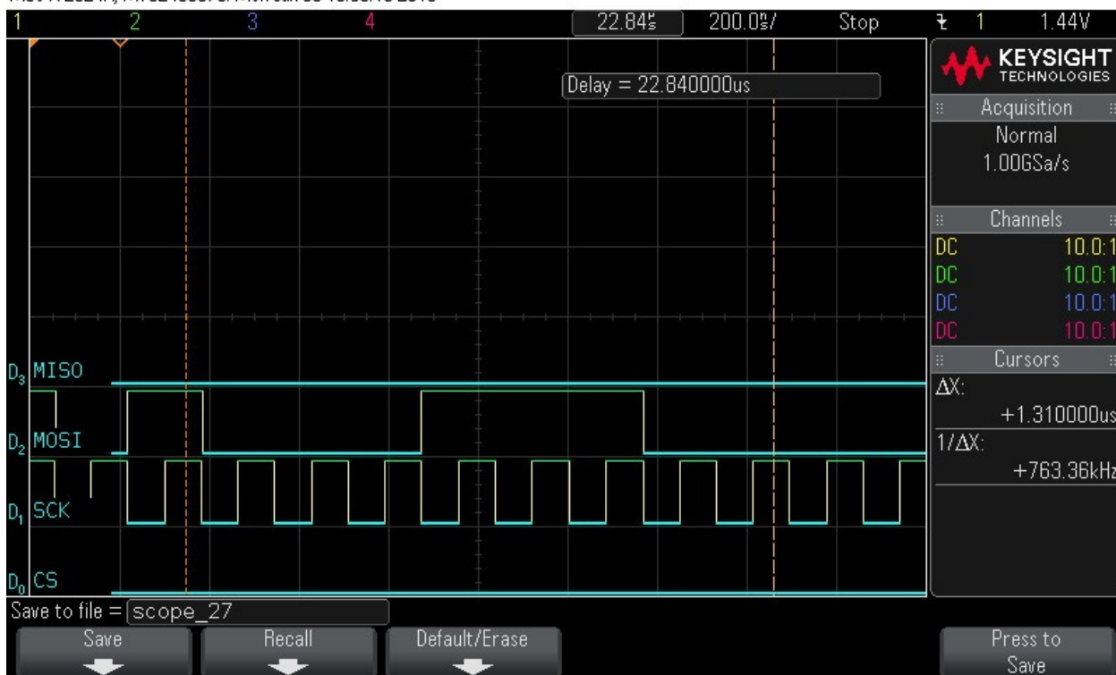
Figure 9-84. Data Byte 2 = 0x1C
