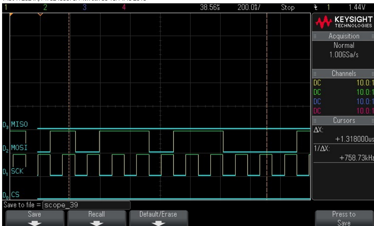
Figure 9-97. Data Byte 15 = 0x62. Note CS signal
