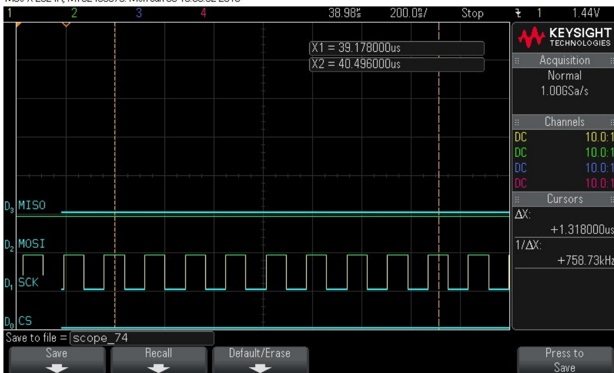
Figure 9-133. Reading Data Byte 13
