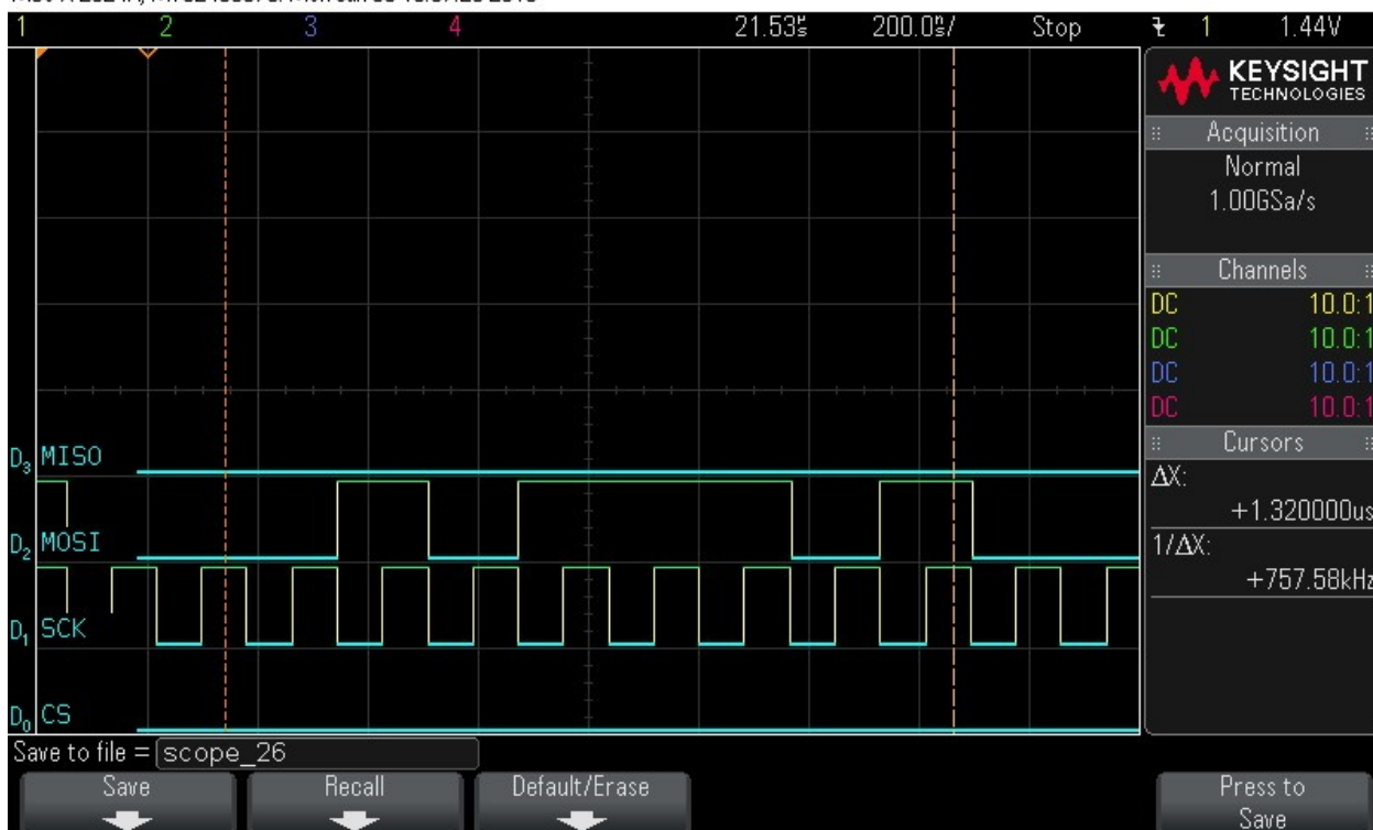
Figure 9-84. Data Byte 2 = 0x1C
