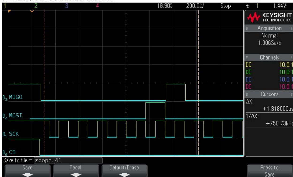
Figure 9-100. Frame Status Command. Command = 0x4. Note CS signal
