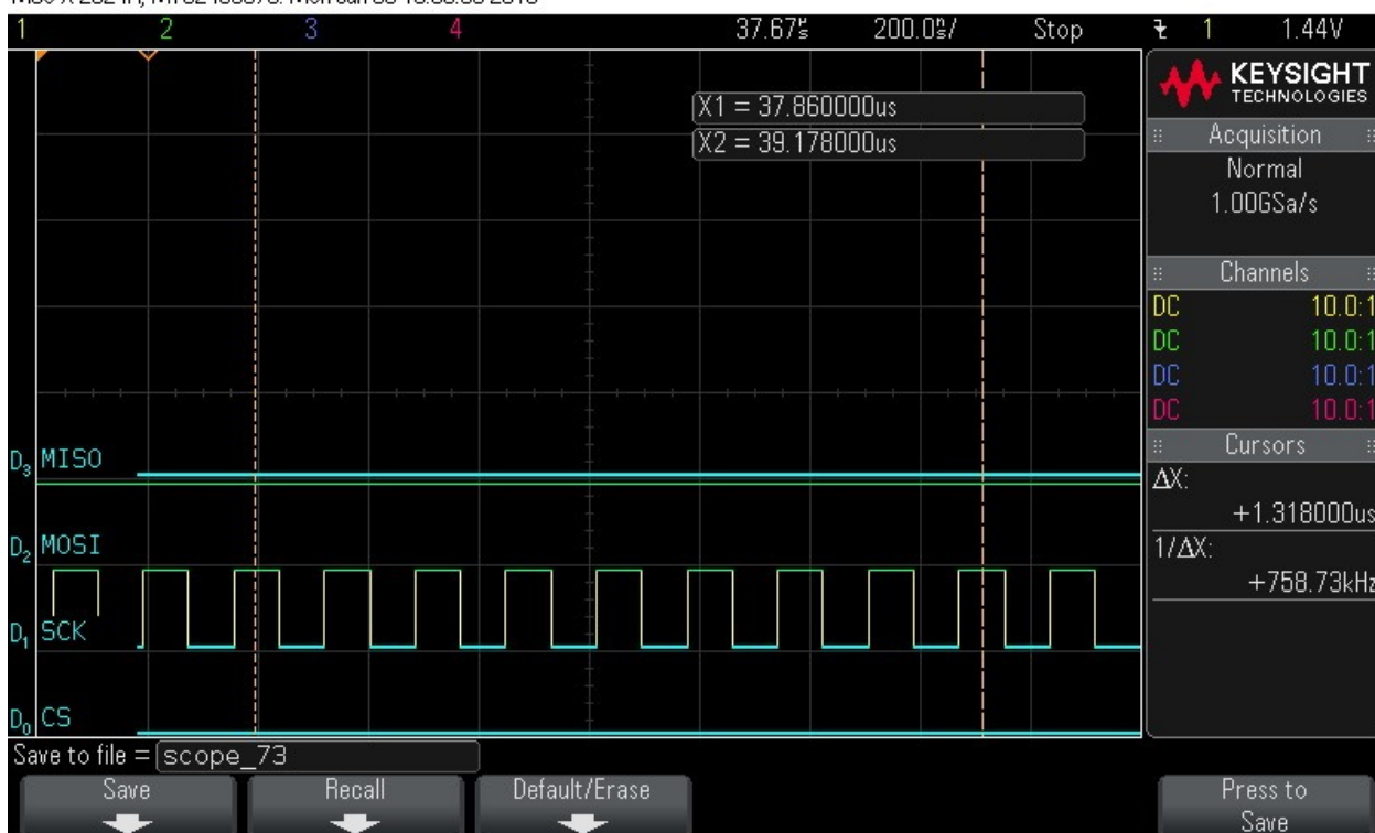
Figure 9-133. Reading Data Byte 13
