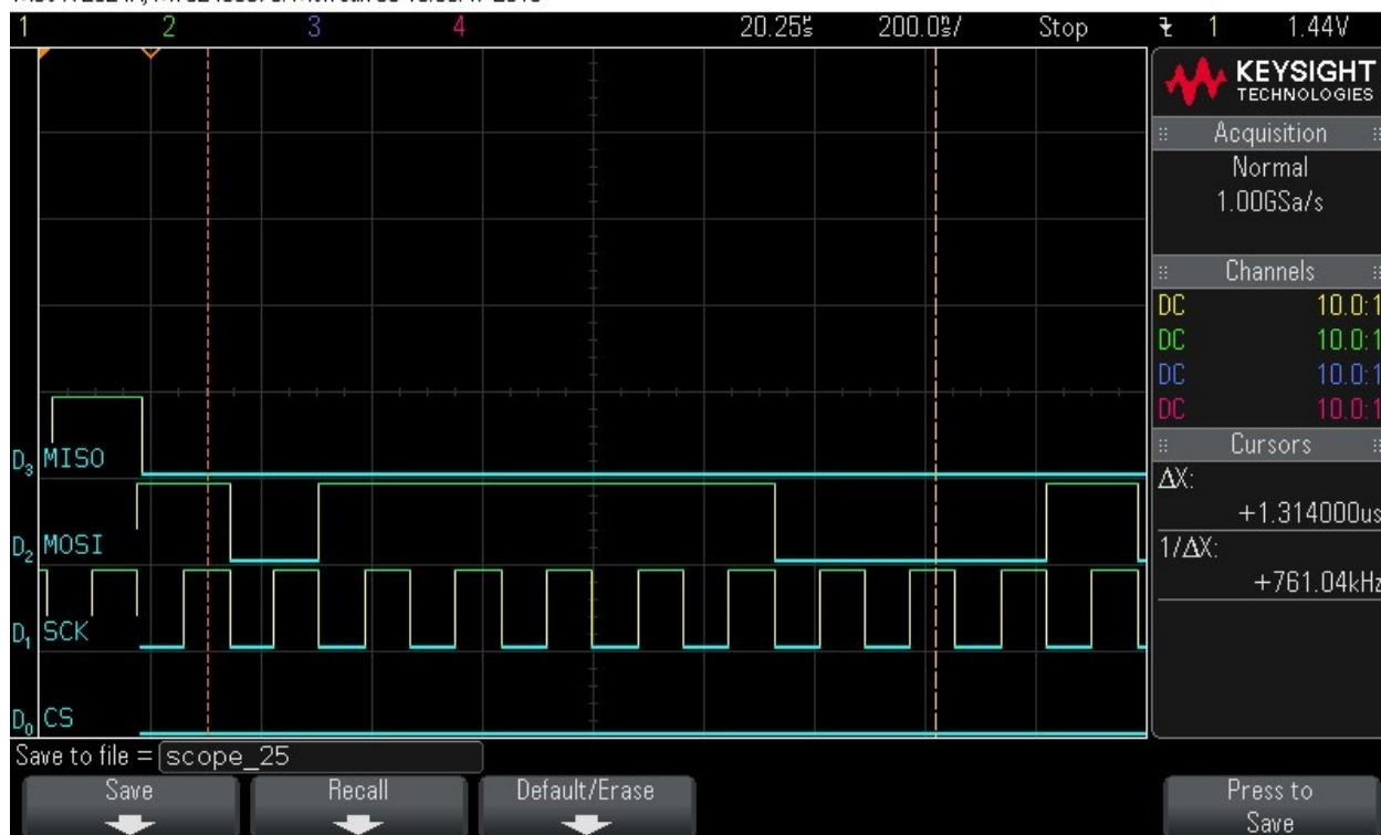
Figure 9-82. Data Byte 0 = 0x7C
