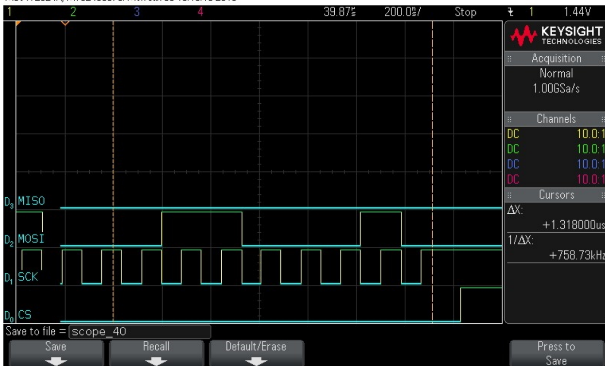
Figure 9-97. Data Byte 15 = 0x62. Note CS signal
