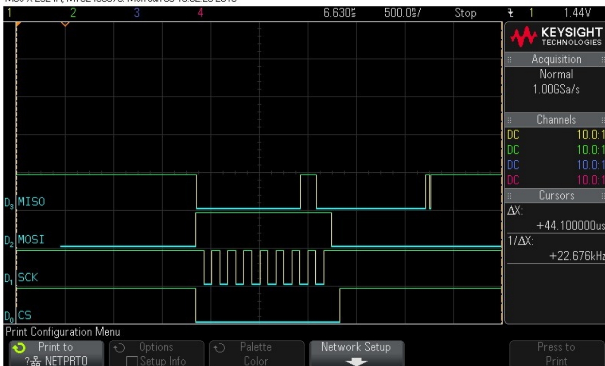
Figure 9-81. Shift in the First Frame. Command = 0x1. Data to Follow. Note CS Signal
