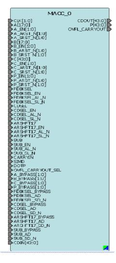
All signals of the SmartFusion2 MACC block, except CDIN and CDOUT, have optional registers. All registers must use the same clock. Each of the registers has enables and resets that can differ from each other. For a complete list of all the block options and their configurations, refer to the Microsemi documentation.
