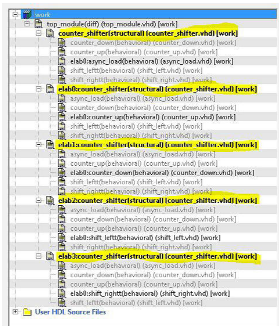
Figure 13-10. Design Hierarchy when an Elaborated Module is Set as root
