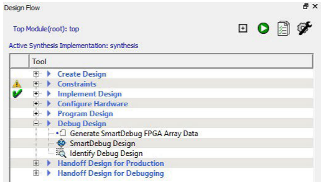
Figure 9-1. Generate SmartDebug FPGA Array Data
