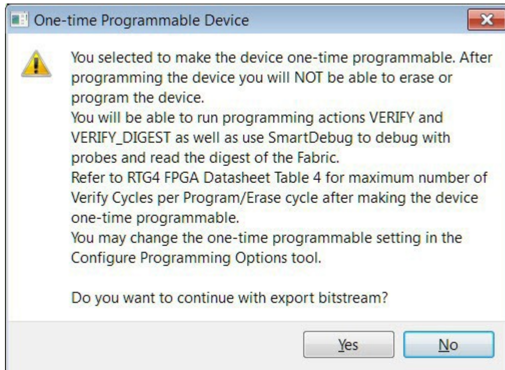
Figure 10-6. One-time Programmable Device Dialog Box
