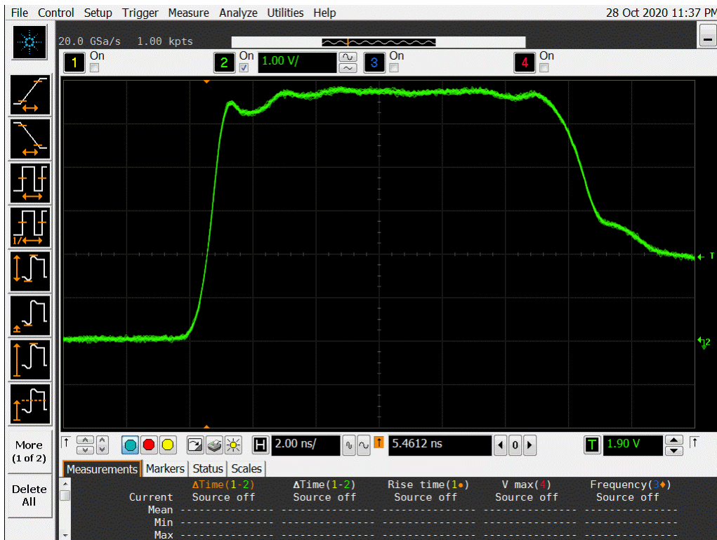
Figure 14b DUT 8601 Post-Annealing Rising Edge
