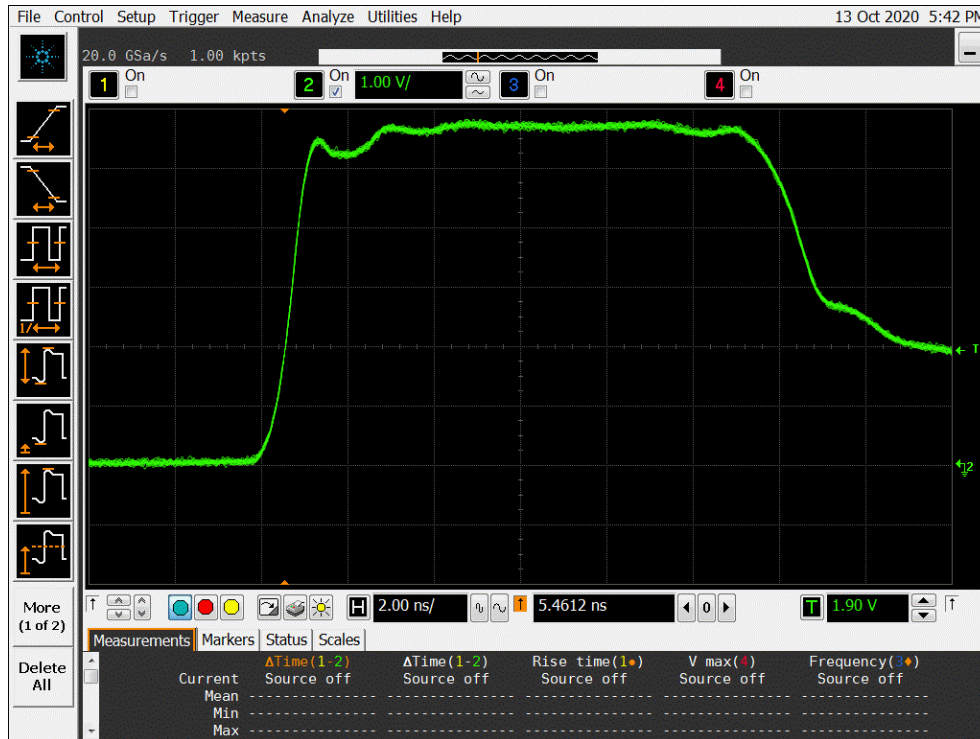
Figure 9a DUT 8626 Pre-Irradiation Rising Edge
