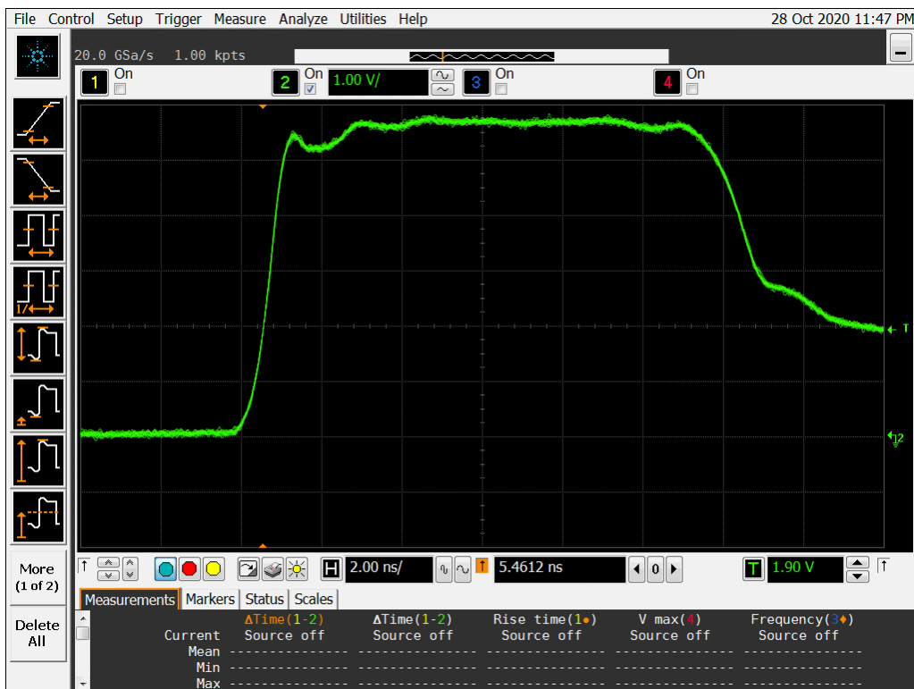
Figure 10b DUT 8628 Post-Annealing Rising Edge
