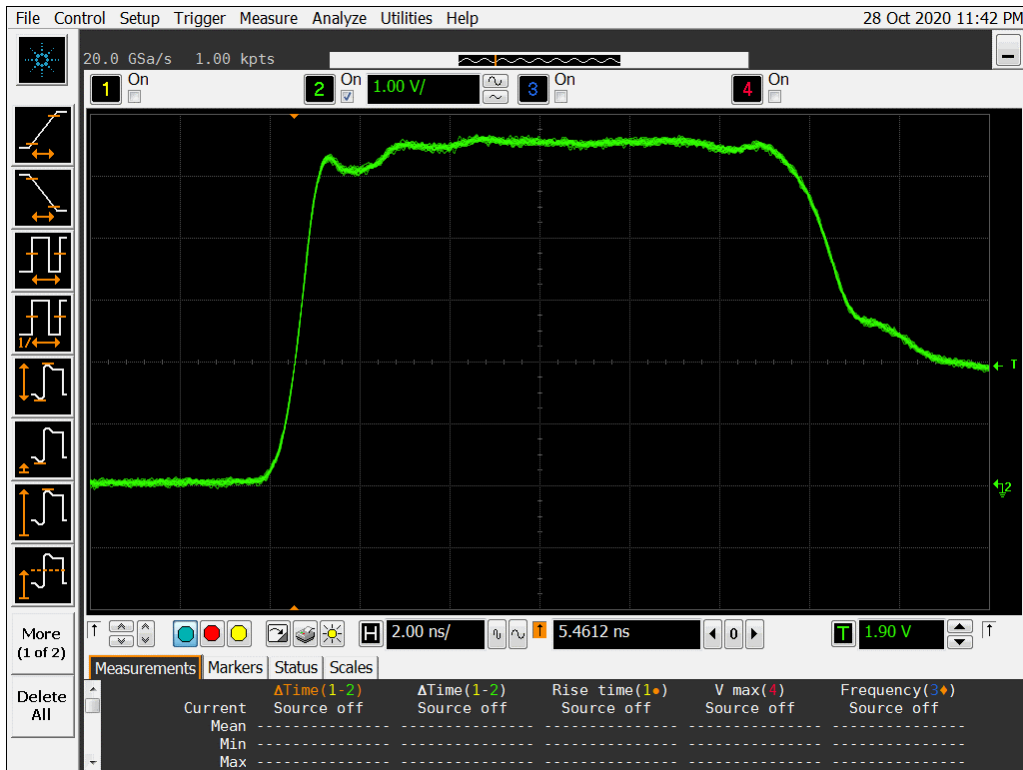
Figure 12b DUT 8623 Post-Annealing Rising Edge
