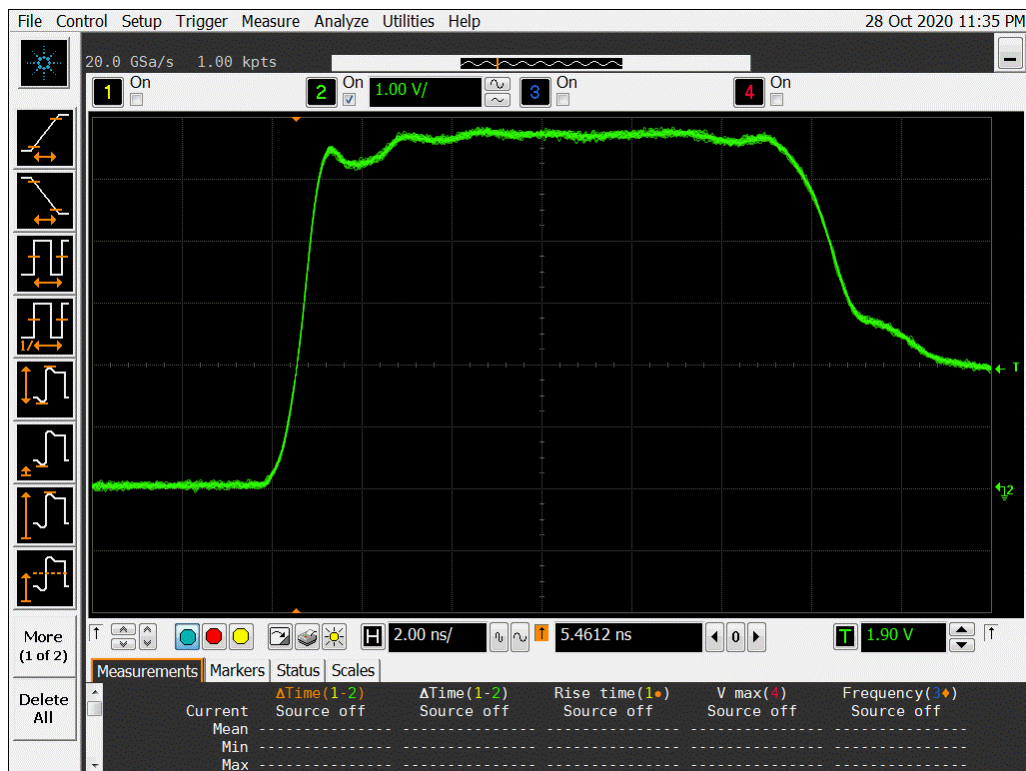
Figure 13b DUT 8593 Post-Annealing Rising Edge
