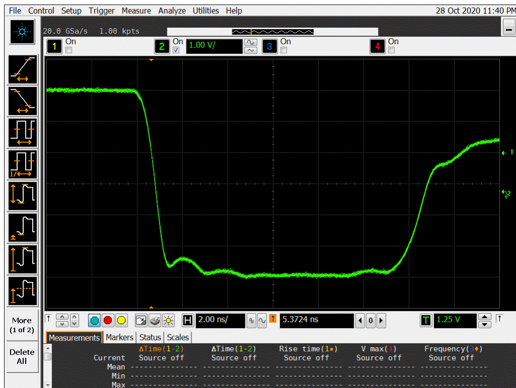
Figure 17b DUT 8605 Post-Annealing Falling Edge
