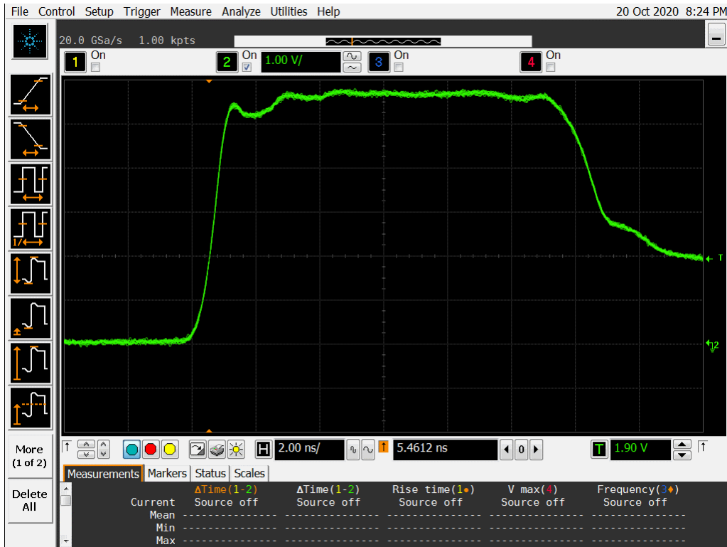
Figure 10a DUT 8690 Pre-Irradiation Rising Edge
