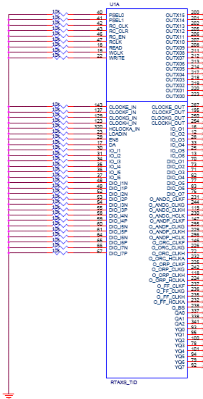
Figure A1 I/O Bias During Irradiation
