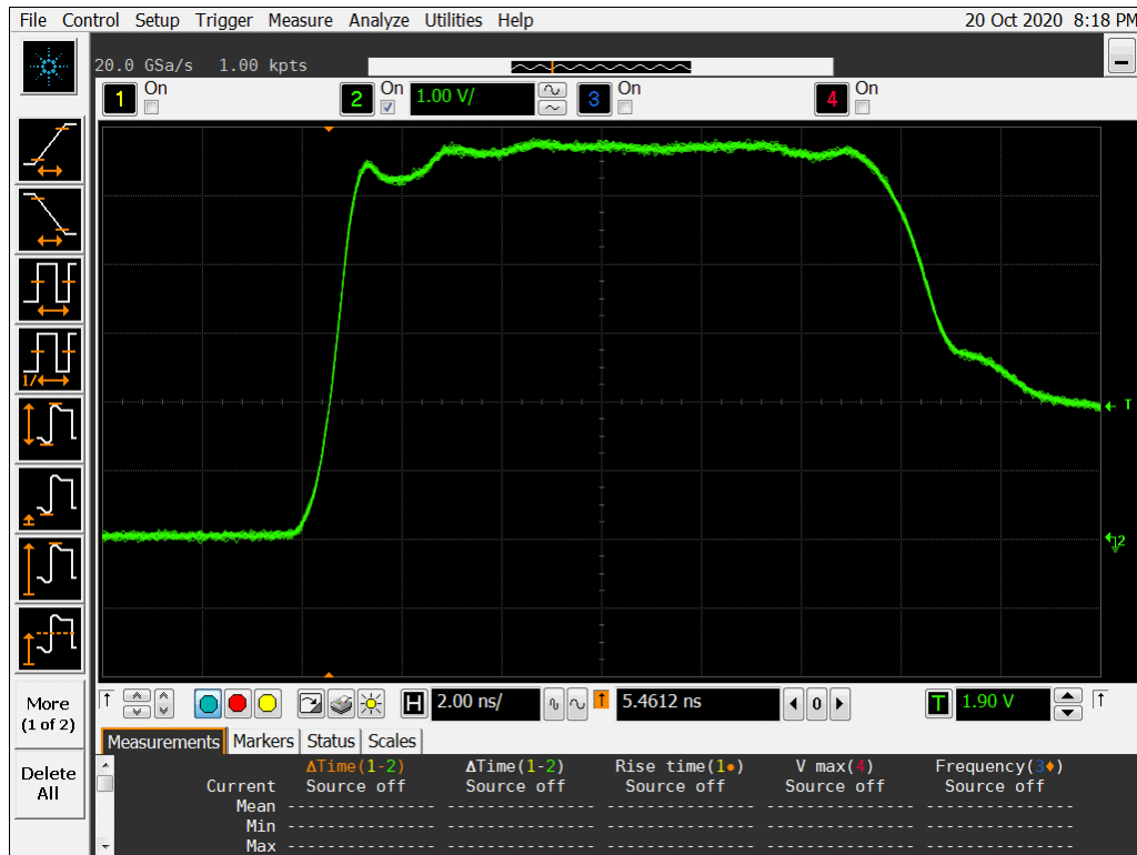
Figure 11a DUT 8662 Pre-Radiation Rising Edge
