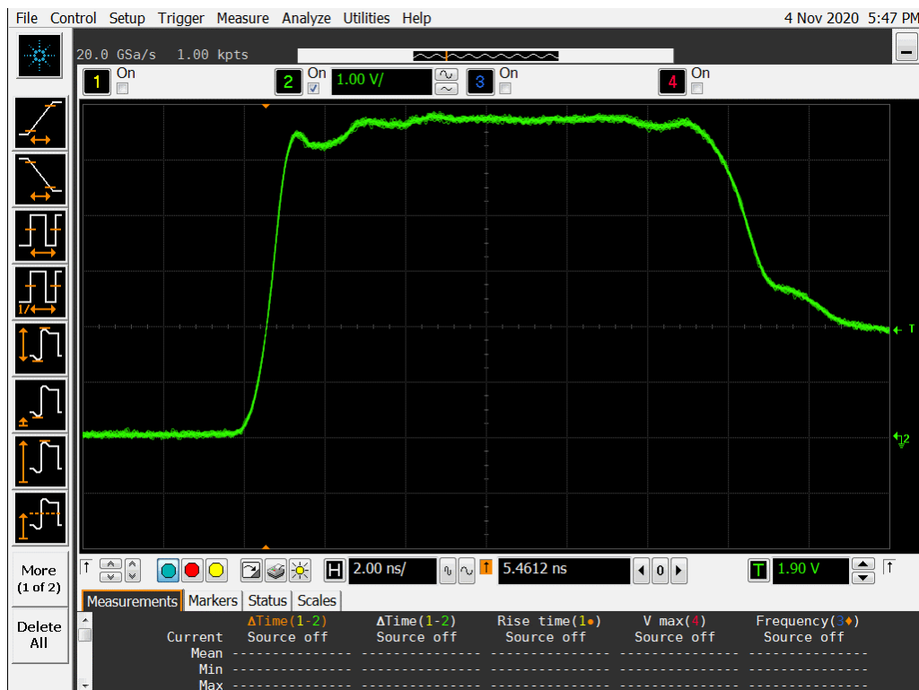
Figure 11b DUT 8662 Post-Annealing Rising edge
