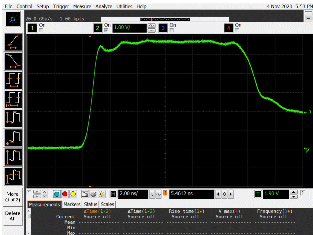
Figure 10b DUT 8690 Post-Annealing Rising Edge
