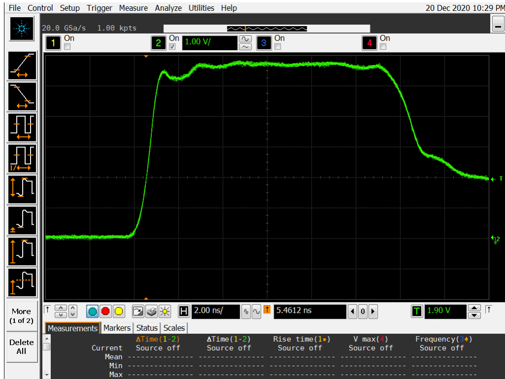
Figure 13a DUT 13260 Pre-Irradiation Rising Edge
