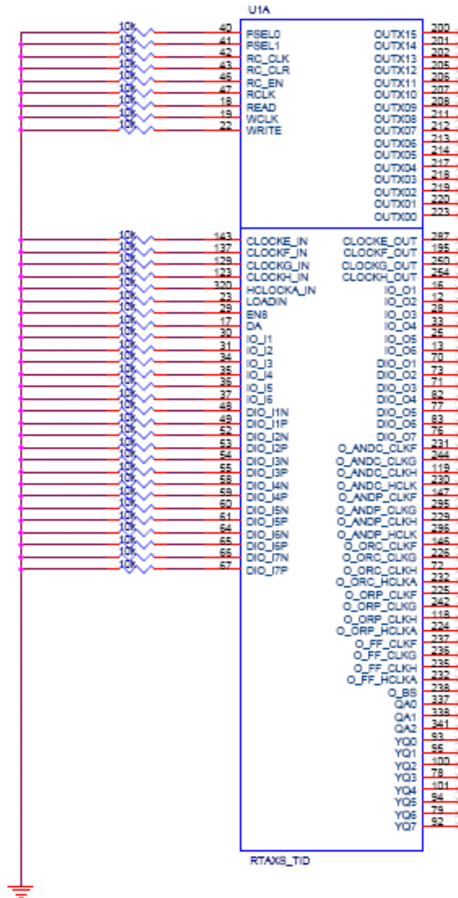
Figure A1 I/O Bias During Irradiation
