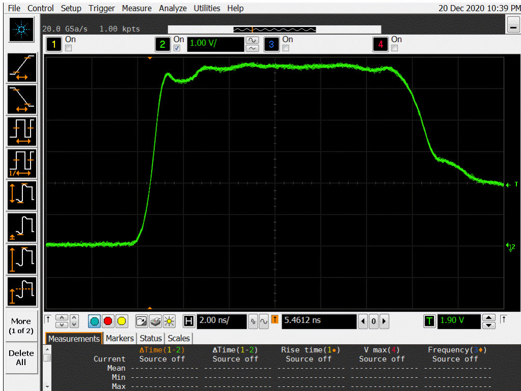
Figure 10a DUT 13304 Pre-Irradiation Rising Edge
