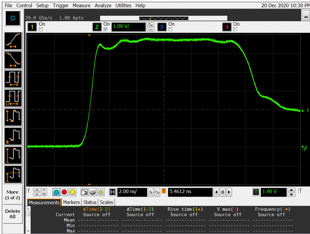
Figure 14a DUT 13267 Pre-Irradiation Rising Edge
