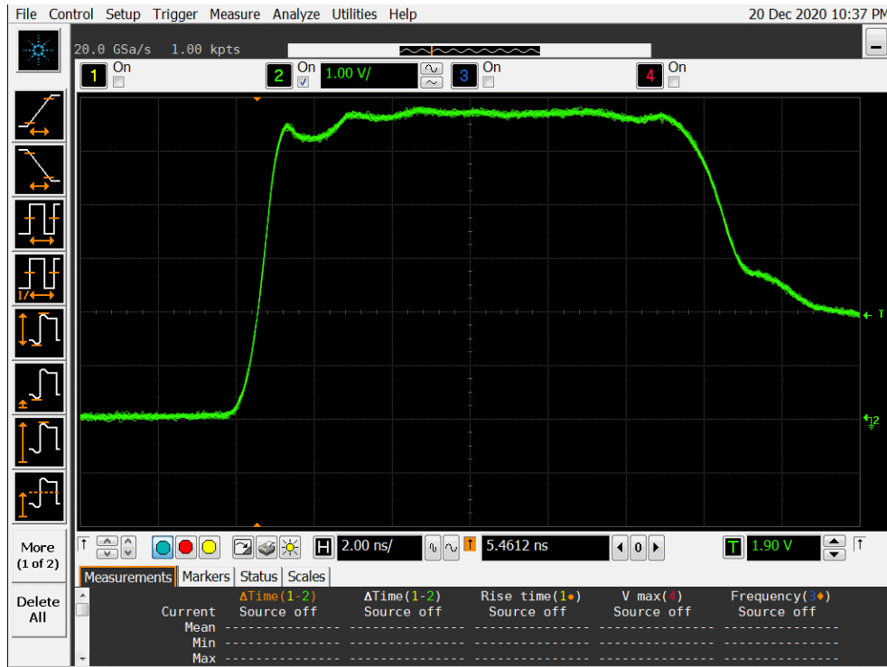
Figure 9a DUT 13298 Pre-Irradiation Rising Edge
