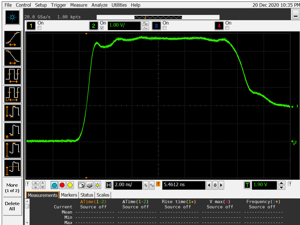
Figure 12a DUT 13280 Pre-Irradiation Rising Edge
