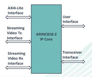
iW ARINC818-2 IP core is compatible with the ARINC818-2 specification. The core supports AXI4-Lite register interface, Streaming Video Tx interface, Streaming Video Rx interface, Transceiver interface and User interface. The ARINC818-2 IP core can be implemented on any transceiver based FPGA.
