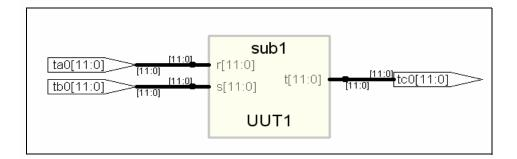
In the figure above, the component declaration has more ports (ext\_1 ext\_2) than entity sub1. The component is synthesized based on the number of ports on the entity.
