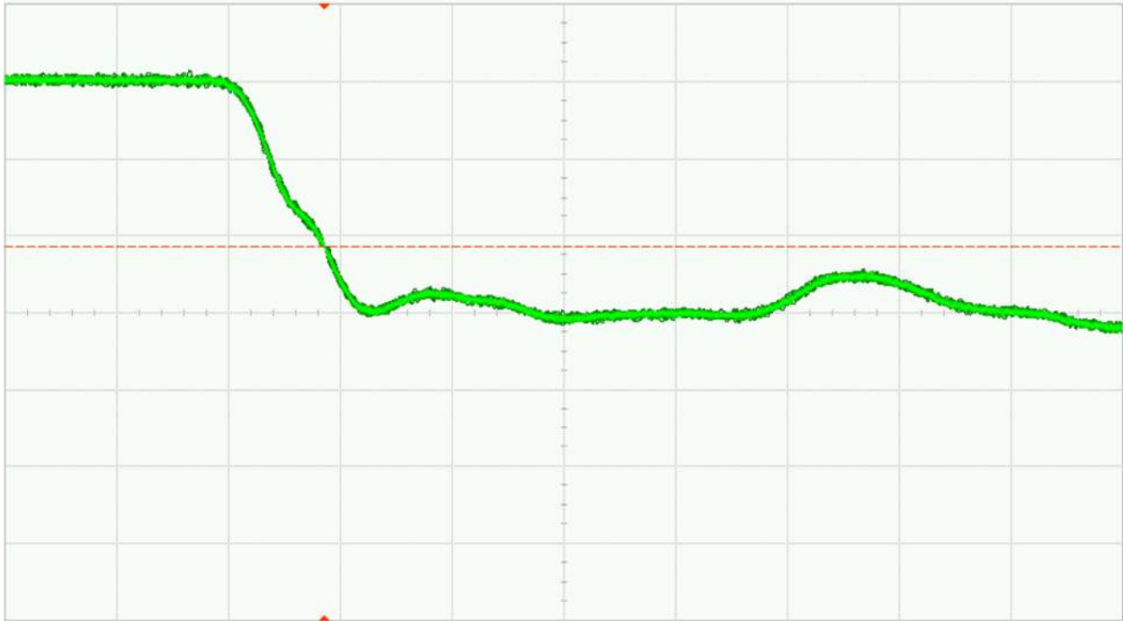
Fig. 29 (a). DUT 10772 pre-irradiation falling edge, abscissa scale is 1V/div and ordinate scale is 2ns/div
