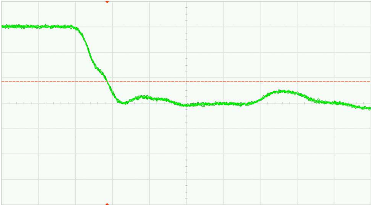
Fig. 30 (a). DUT 10807 pre-irradiation falling edge, abscissa scale is 1V/div and ordinate scale is 2ns/div
