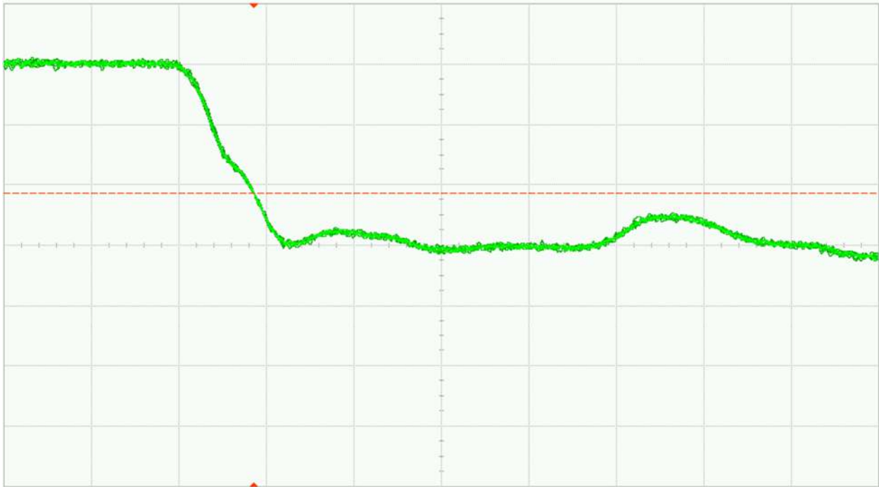
Fig. 29 (b). DUT 10772 post-annealing falling edge, abscissa scale is 1V/div and ordinate scale is 2ns/div
