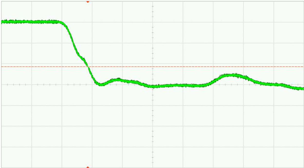
Fig. 28 (b). DUT 10765 post-annealing falling edge, abscissa scale is 1V/div and ordinate scale is 2ns/div
