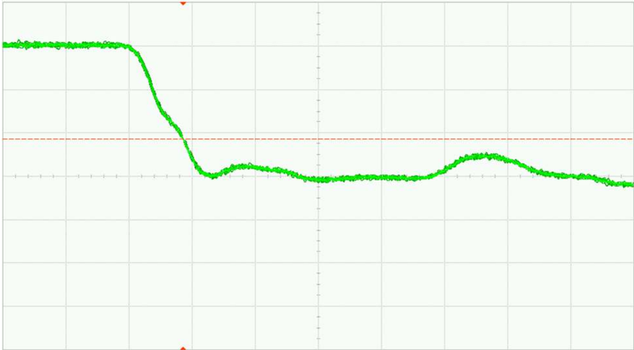
Fig. 27 (a). DUT 10759 pre-irradiation falling edge, abscissa scale is 1V/div and ordinate scale is 2ns/div
