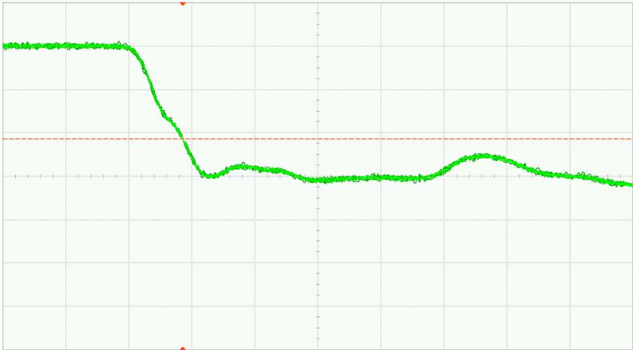
Fig. 27 (b). DUT 10759 post-annealing falling edge, abscissa scale is 1V/div and ordinate scale is 2ns/div
