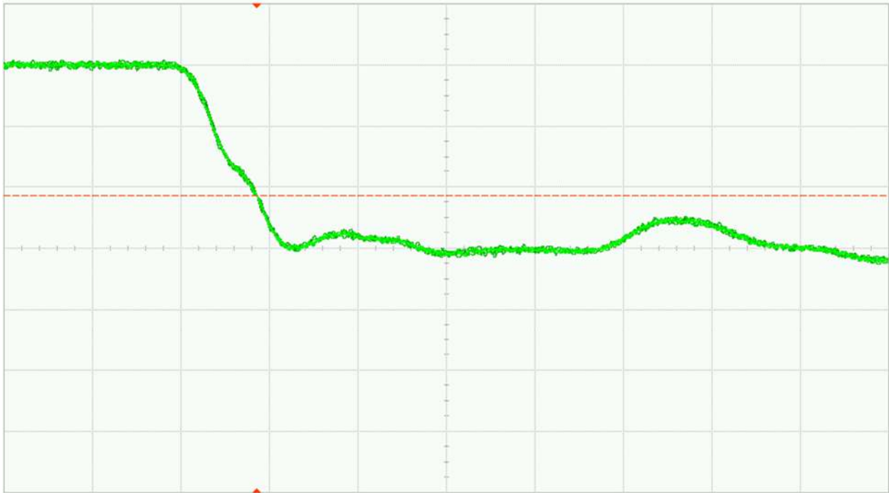
Fig. 30 (b). DUT 10807 post-annealing falling edge, abscissa scale is 1V/div and ordinate scale is 2ns/div
