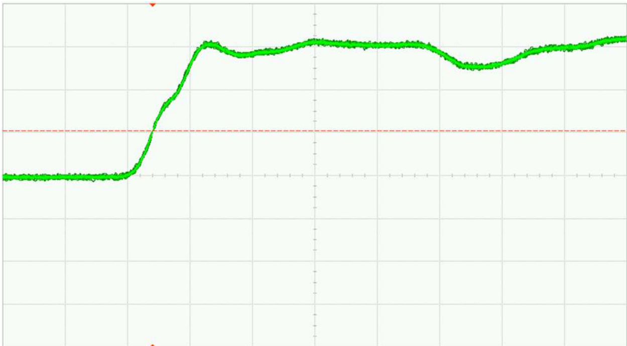
Fig. 26 (b). DUT 10822 post-annealing rising edge, abscissa scale is 1V/div and ordinate scale is 2ns/div
