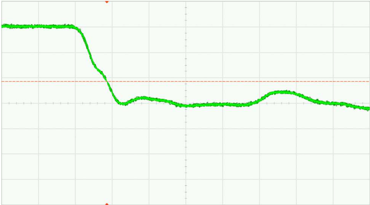
Fig. 31 (a). DUT 10822 pre-irradiation falling edge, abscissa scale is 1V/div and ordinate scale is 2ns/div
