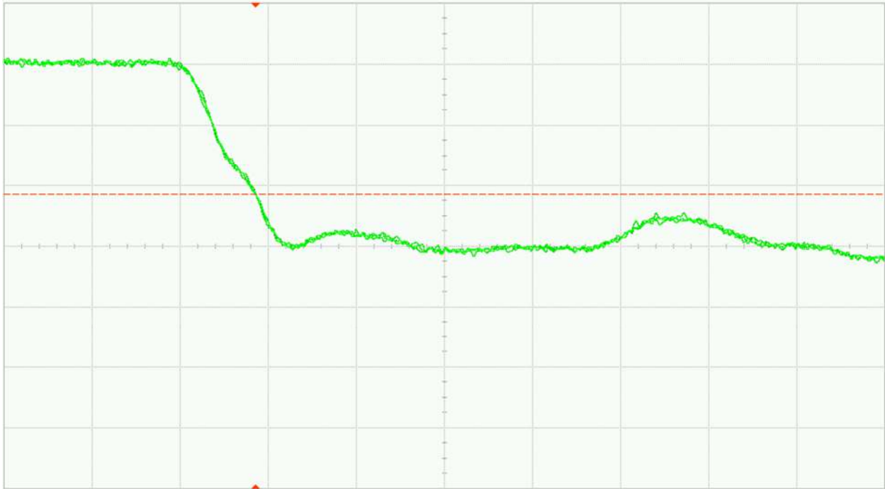
Fig. 28 (a). DUT 10765 pre-irradiation falling edge, abscissa scale is 1V/div and ordinate scale is 2ns/div
