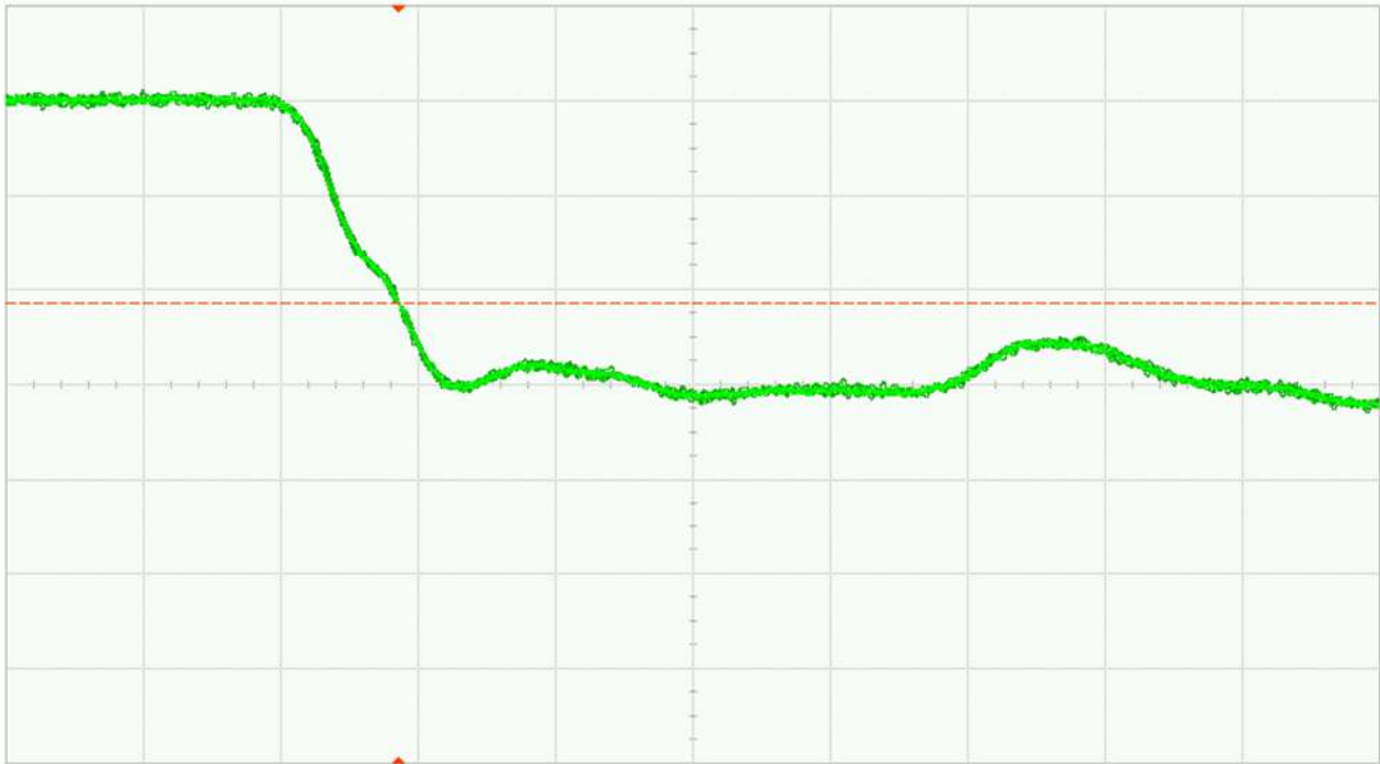
Fig. 31 (b). DUT 10822 post-annealing falling edge, abscissa scale is 1V/div and ordinate scale is 2ns/div
