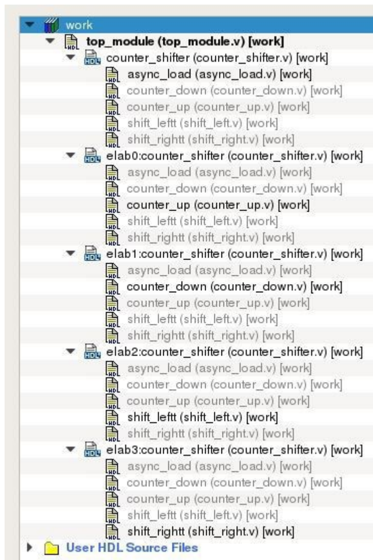
Figure 11-17. Design Hierarchy with Elaborated Modules (Verilog)
