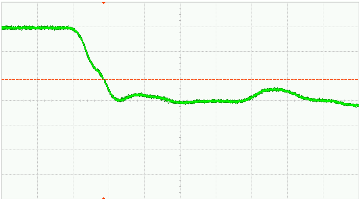
Fig. 36 (a). DUT 4017 pre-irradiation Falling edge, abscissa scale is 1V/div and ordinate scale is 2ns/div
