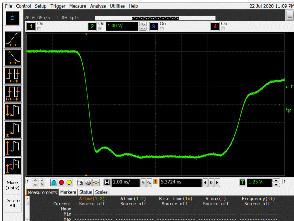
Figure 19b DUT 13964 Post-Annealing Falling Edge
