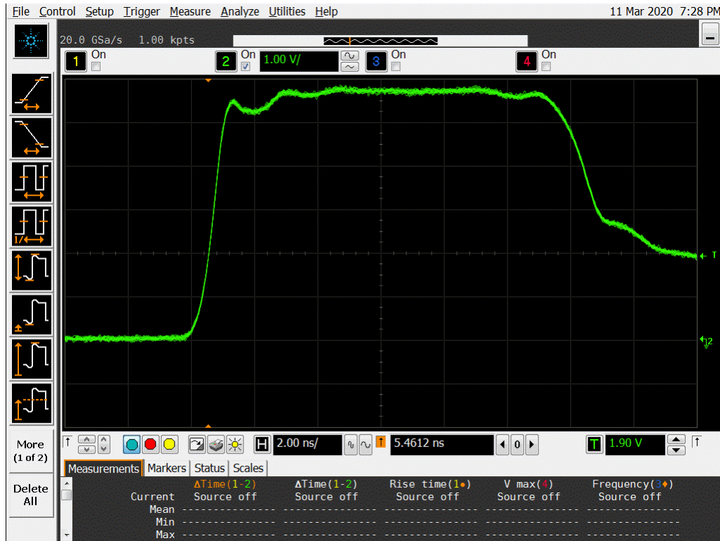
Figure 13a DUT 13964 Pre-Irradiation Rising Edge
