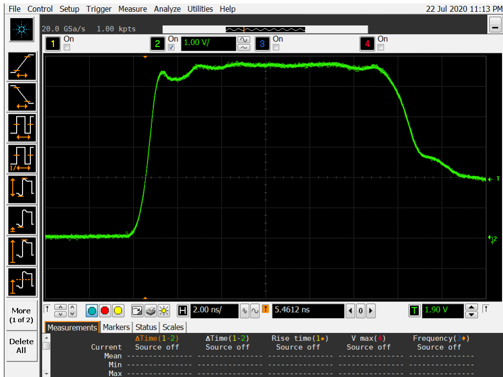
Figure 11b DUT 13992 Post-Annealing Rising edge
