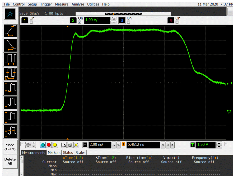
Figure 9a DUT 14004 Pre-Irradiation Rising Edge
