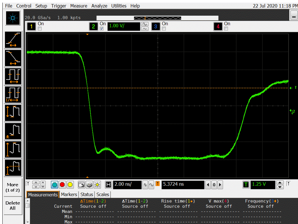
Figure 15b DUT 14004 Post-Annealing Falling Edge
