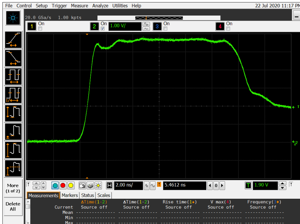
Figure 9b DUT 14004 Post-Annealing Rising Edge
