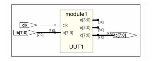
In the figure above, the entity module1 has extra ports a and e that are not defined in the corresponding component declaration mod1. The additional ports are not connected during synthesis.
