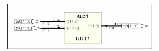
In the figure above, the component declaration has more ports (ext\_1 ext\_2) than entity sub1. The component is synthesized based on the number of ports on the entity.
