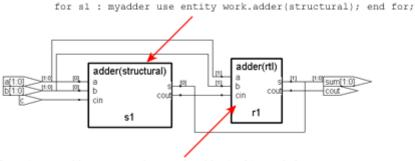
for r1 : myadder use entity work.adder(rtl); end for;
