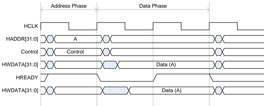
**Figure 3 AHB Transfer with One Wait State**
