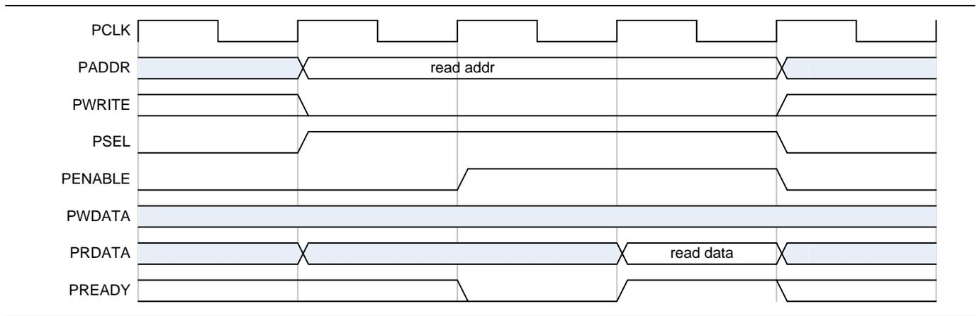
**Figure 7** APB Read Transfer with One State
