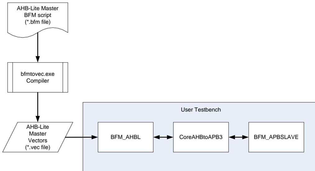
**Figure 10** CoreAHBtoAPB3 User Testbench
