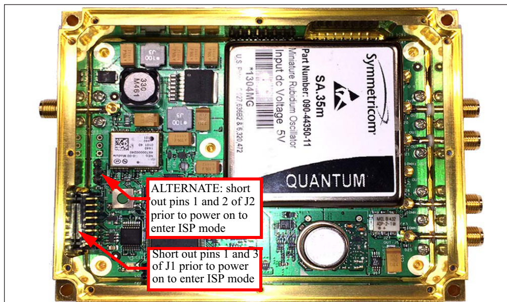
FIGURE 4-1: Location of Header J2 Internally to the Enclosure.
