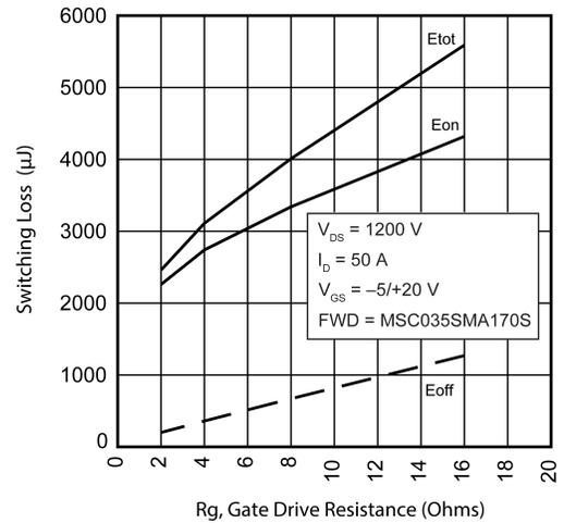
Figure 14 • Switching Energy vs. R<sub>g</sub>
