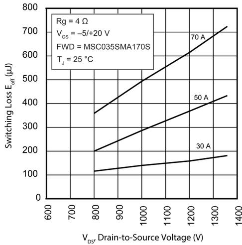
Figure 13 • Switching Energy E<sub>off</sub> vs. V<sub>DS</sub> & I<sub>D</sub>
