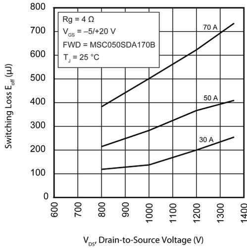
Figure 17 • Switching Energy  $E_{off}$  vs.  $V_{DS}$  and  $I_D$
