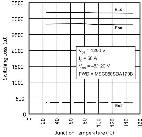
Figure 19 • Switching Energy vs.  $T_j$
