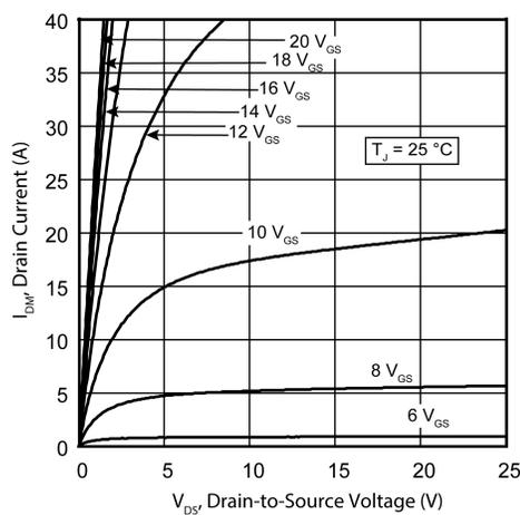
**Figure 2 • Drain Current vs.  $V_{DS}$**
