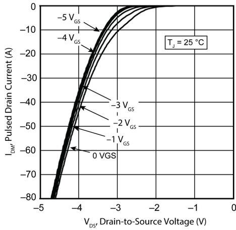
Figure 9 •  $I_{DM}$  vs.  $V_{DS}$  3<sup>rd</sup> Quadrant Conduction
