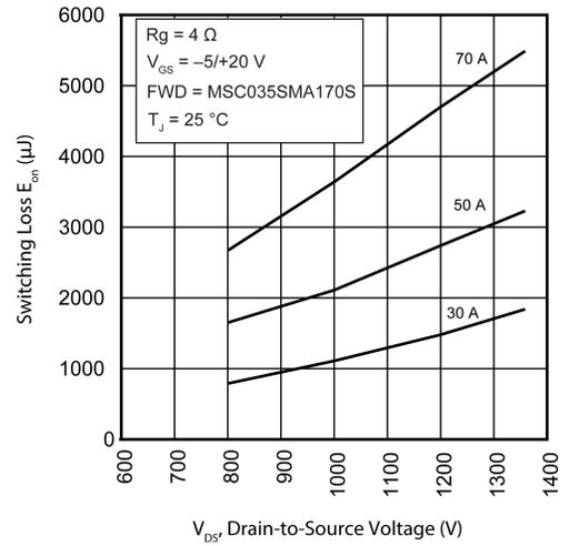
Figure 12 • Switching Energy E<sub>on</sub> vs. V<sub>DS</sub> and I<sub>D</sub>
