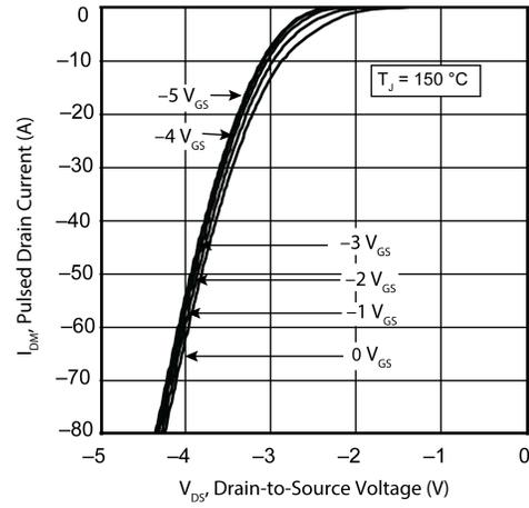
Figure 10 •  $I_{DM}$  vs.  $V_{DS}$  3<sup>rd</sup> Quadrant Conduction
