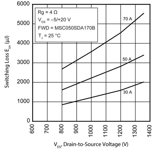
Figure 16 • Switching Energy  $E_{on}$  vs.  $V_{DS}$  and  $I_D$
