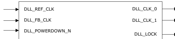
Figure 37 • DLL Ports—Clock Injection Delay Removal Mode
