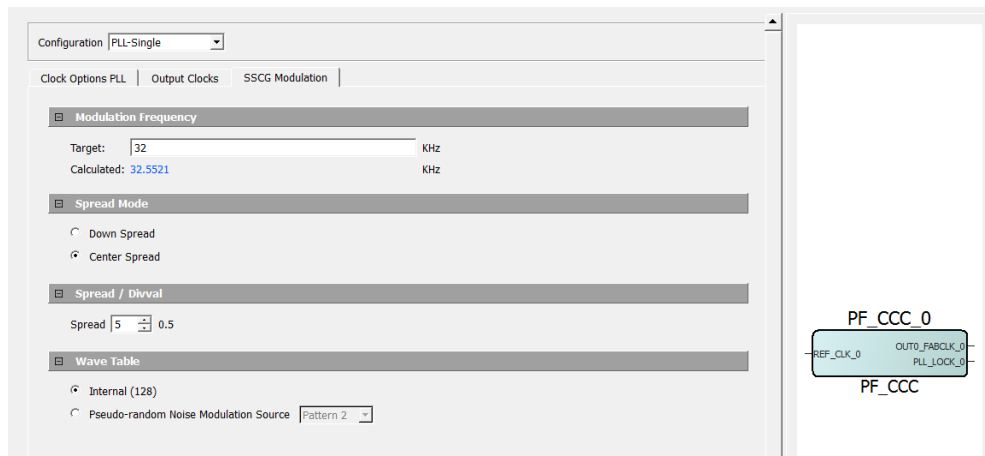
Figure 43 • PLL-Single Configuration—SSCG Modulation
