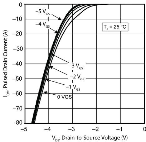
Figure 9 •  $I_{DM}$  vs.  $V_{DS}$  3<sup>rd</sup> Quadrant Conduction
