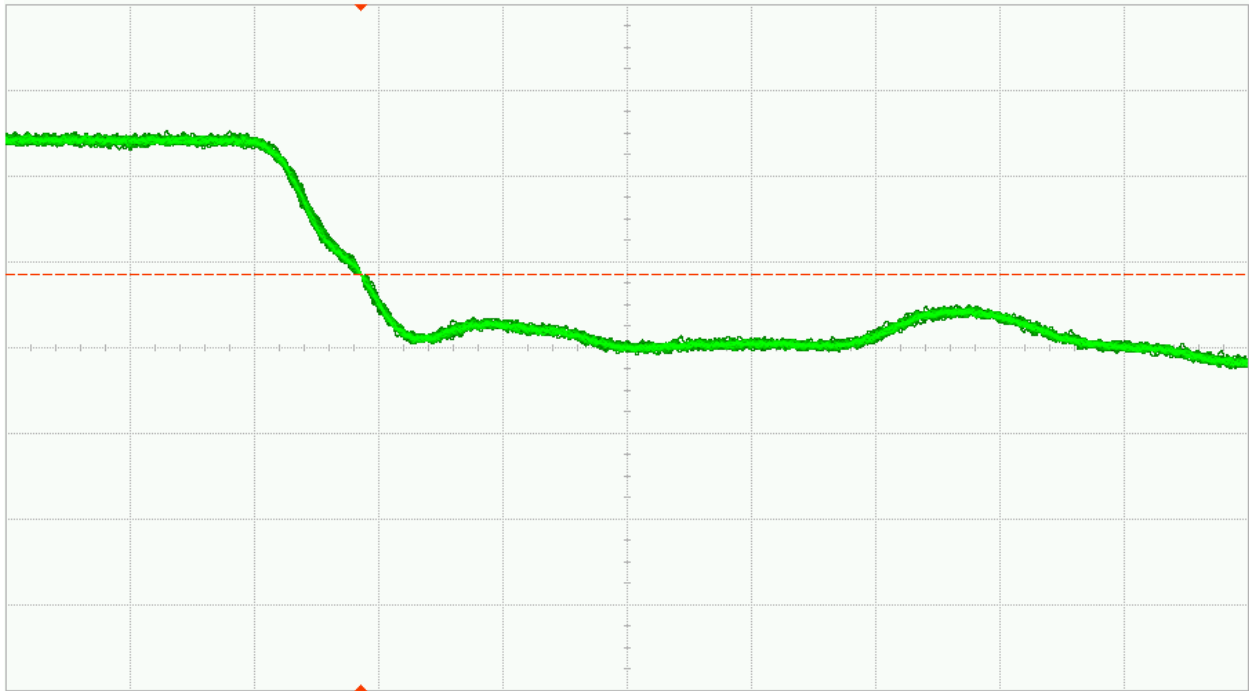
Fig. 36 (a). DUT 05072 pre-irradiation falling edge, abscissa scale is 1V/div and ordinate scale is 2ns/div
