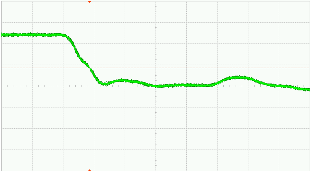
Fig. 37 (a). DUT 05094 pre-irradiation falling edge, abscissa scale is 1V/div and ordinate scale is 2ns/div
