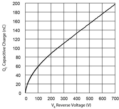
Figure 6 • Total Capacitive Charge vs.  $V_R$
