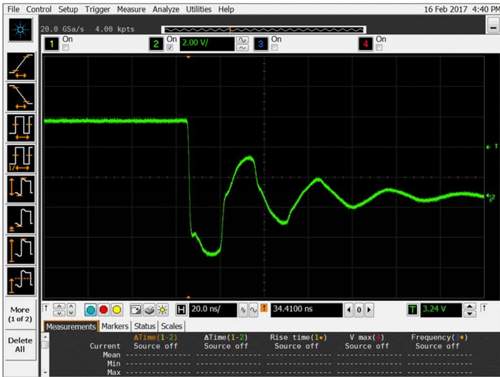
Figure 16b DUT 11255 Post-Annealing Falling Edge
