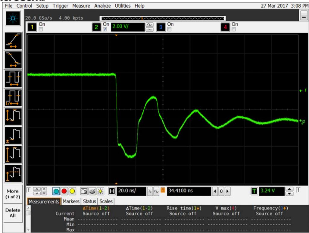
Figure 19a DUT 11048 Pre-Irradiation Falling Edge
