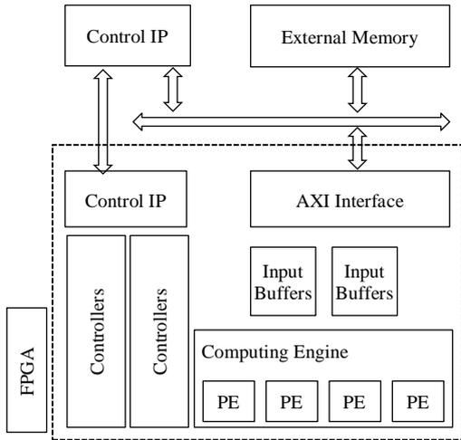
Fig. 7: CDL FPGA Core Interface
