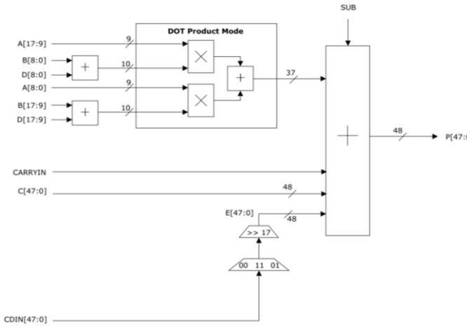
Fig. 2. DOTP Mode available in PolarFire FPGA's Math block.
