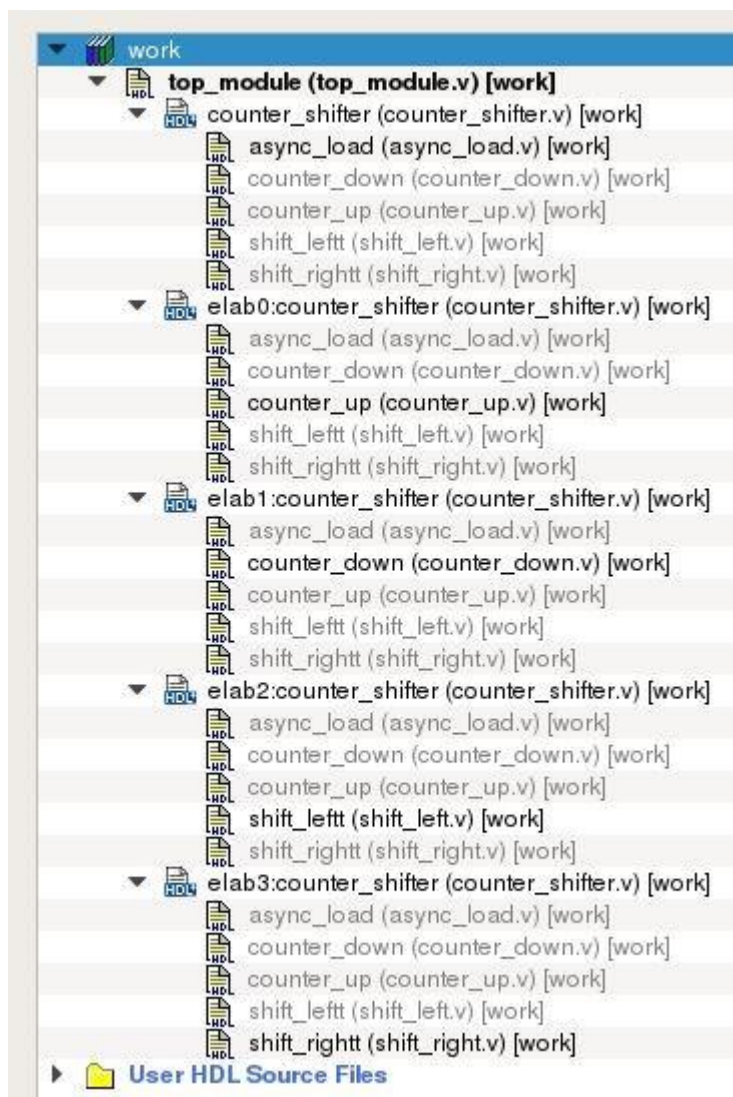
Figure 115 · Design Hierarchy with Elaborated modules(Verilog)
