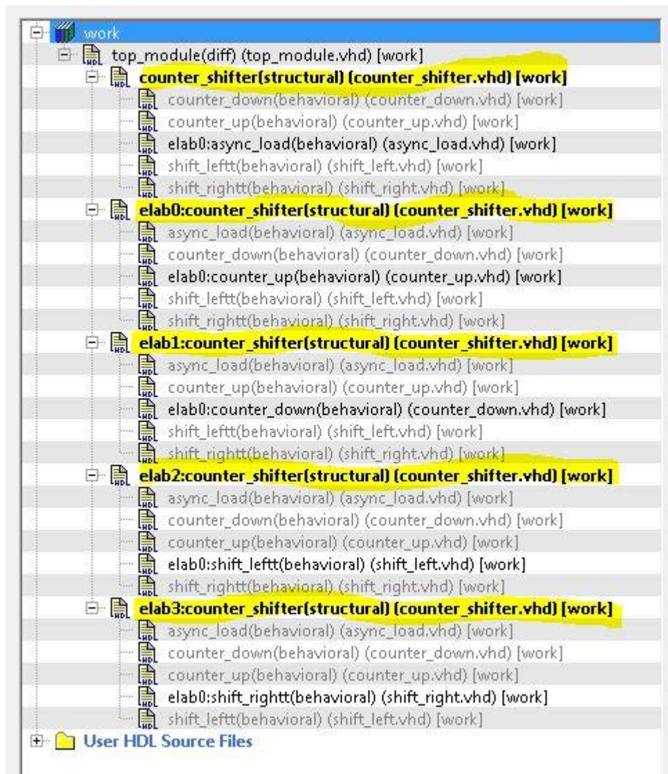
Figure 117 • Design Hierarchy when one of the elaborated module is set as root
