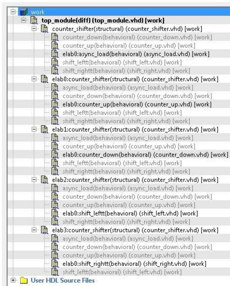
Figure 116 · Design Hierarchy with Elaborated modules(VHDL)
