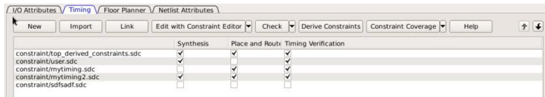
Figure 24 · Timing Constraints SDC file and Tool Association
