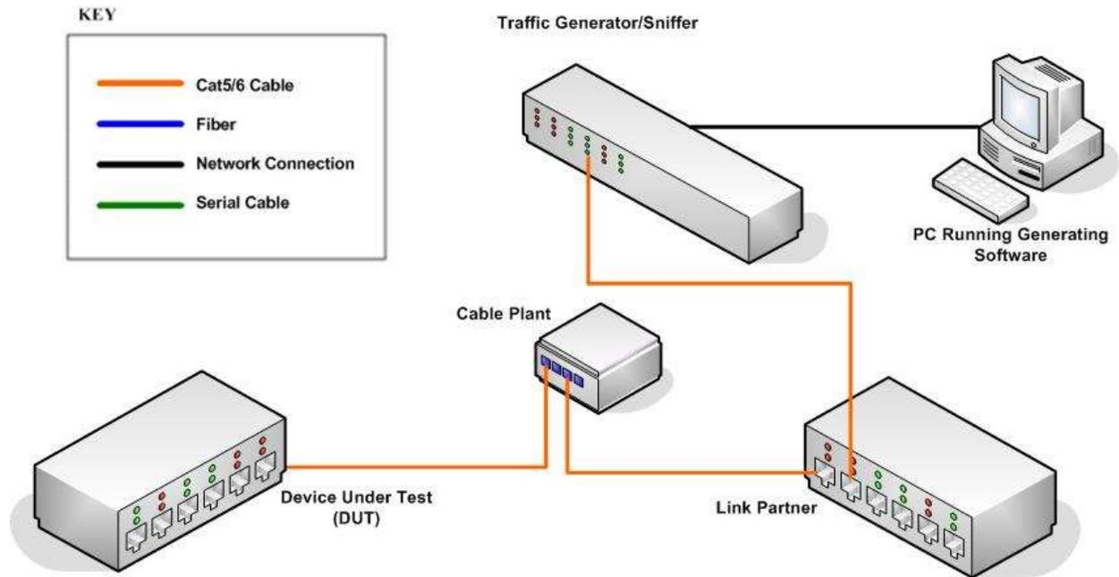
Figure 1 - Test Configuration
