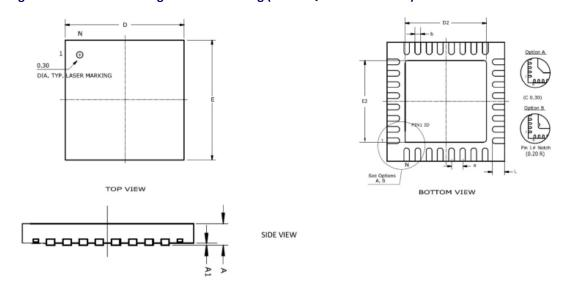
The following table lists the dimensions and measurements of the PD69210 package.
