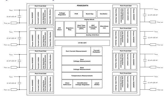
The following sections describe the functional blocks of the PD69204T4 device.
