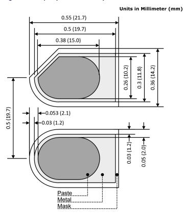
**Note**: The CM has latitude to modify the solder paste stencil for manufacturability reasons. The solder paste stencil covers 65% to 80% of the thermal pad, and must not allow solder to be applied to the thermal vias under the QFN package, using an appropriate method. Any design should be subject to system validation and qualification, prior to commitment to mass production of field deployment. A 5 mm stencil is used.
