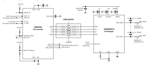
**Note**: Consult Microsemi AN240 Designing an IEEE 802.3af/802.3at/802.3bt-Compliant PD69208 48-Port PoE System (Document Number: PD-000359851) for complete reference design.
