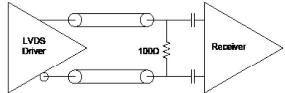
**Figure 6. LVDS to LVDS Connection, Internal 100ohm Resistor**
