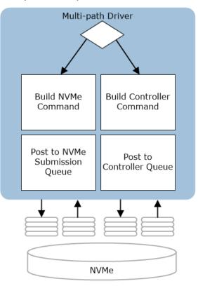
To determine which path to use, the driver performs a few lightweight checks such as:
