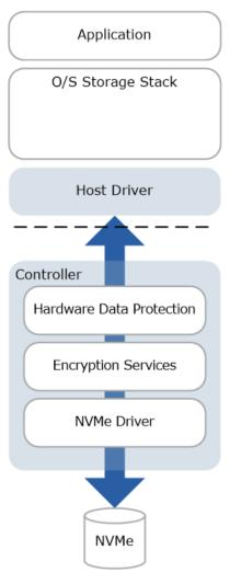
Traditional hardware RAID controllers offload host compute and memory resource consumption from the host but the controller is always present in the path to the drive, even in situations where offloads are not required. For example, writes that require parity generation need to be routed through the controller to take advantage of the offload but a read to the same logical volume would be lower latency if it could be issued from the host straight to the drive.
