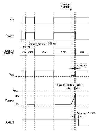
The delay time is controlled by R31 and C17. ADuM4136 has a blanking time of 300 ns, which should be enough for a SiC power stage in most cases. The additional delay past blanking can be increased by adding C17 or decreased slightly by reducing R31. If a scope is used to observe the desat signal at the input to the ADuM4135, the low-side driver should be observed and a very low capacitance probe should be used.
