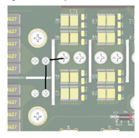
Figure 7 • Singled-ended Input Connection
