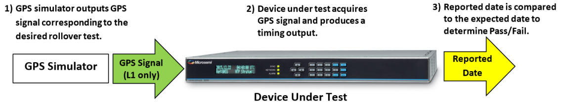
Figure 2 • Equipment Setup for GPS Week Rollover Testing
