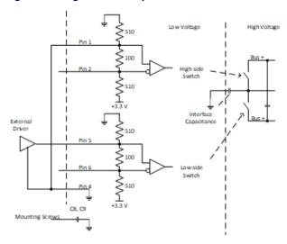
Figure 8 • Differential Input Connection
