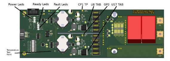
The PCB is shipped configured for -5 V, 20 V gate drive. R82 and R37 should be shorted to yield -5 V, 18 V gate drive. Four test points are shown in the above diagram CP1 to U8 tab should be 25 V when configured for 20 V gate drive and 23 V with 18 V gate drive. U8 tab to the corresponding module source lead should measure 5 V. On the low side test point GP2 and U17 tab have the same role.
