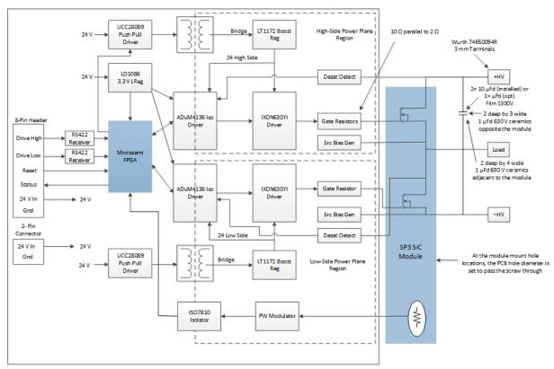
Figure 1 • Block Diagram with Half Bridge
