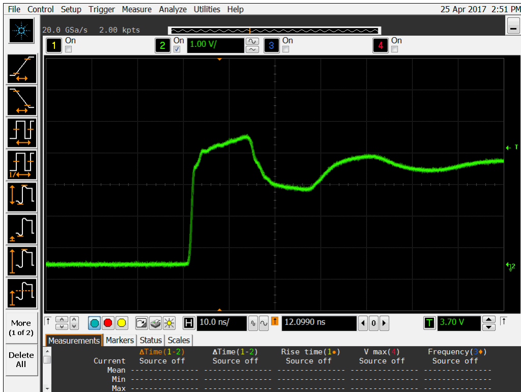
Figure 9b DUT 986 Post-Annealing Rising Edge.
