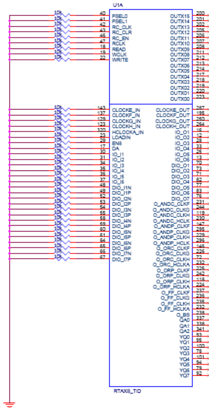
Figure A1 I/O Bias During Irradiation
