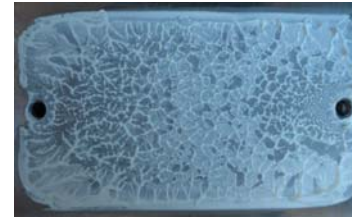
Picture 6: Grease on the heat sink after removing the module
