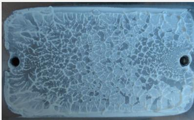
**Figure 2-3. Grease on the Module After Disassembling**
