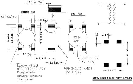
\*\*THE PIN COPLANARITY :0.1 mm MAX (MAX DIMENSION OF 4 TERMINALS - MIN DINENSION OF 4 TERMINALS) \*\*
