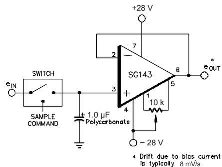
Figure 11 - Low - Drift Sample and Hold
