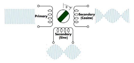
The device used to process the resolver signals and convert them in to a digital angle format is called a resolver to digital converter (RDC). The resolver IP implements the functionality of a RDC. The IP provides excitation signal in the form of a square wave to the primary winding whose frequency can be configured. The IP processes the secondary signals, demodulates them and calculates the angle and speed of the rotor.
