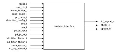
The resolver interface IP generates a square wave that is fed to the primary winding of the resolver. The frequency of the square wave can be configured through hf\_sig\_period\_i input. The cos\_i and sin\_i signals from the secondary windings are demodulated and filtered to get effective cosine and sine signals. A phase-locked loop (PLL) is used to extract angle and speed from cosine and sine signals.
