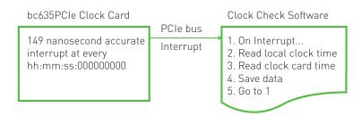
FIG 4 Clock Check Software Loop
