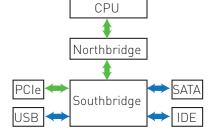
FIG 3 Location of the PCIe card/bus relative to the CPU running software applications
