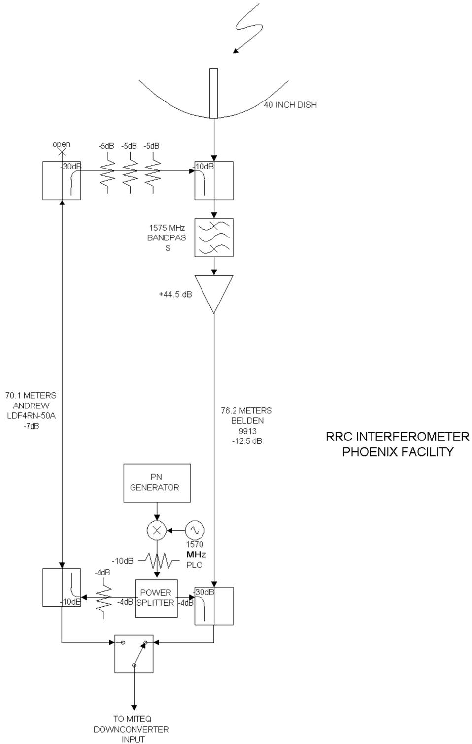
FIG.3 L-Band RF and Calibration Subsystem
