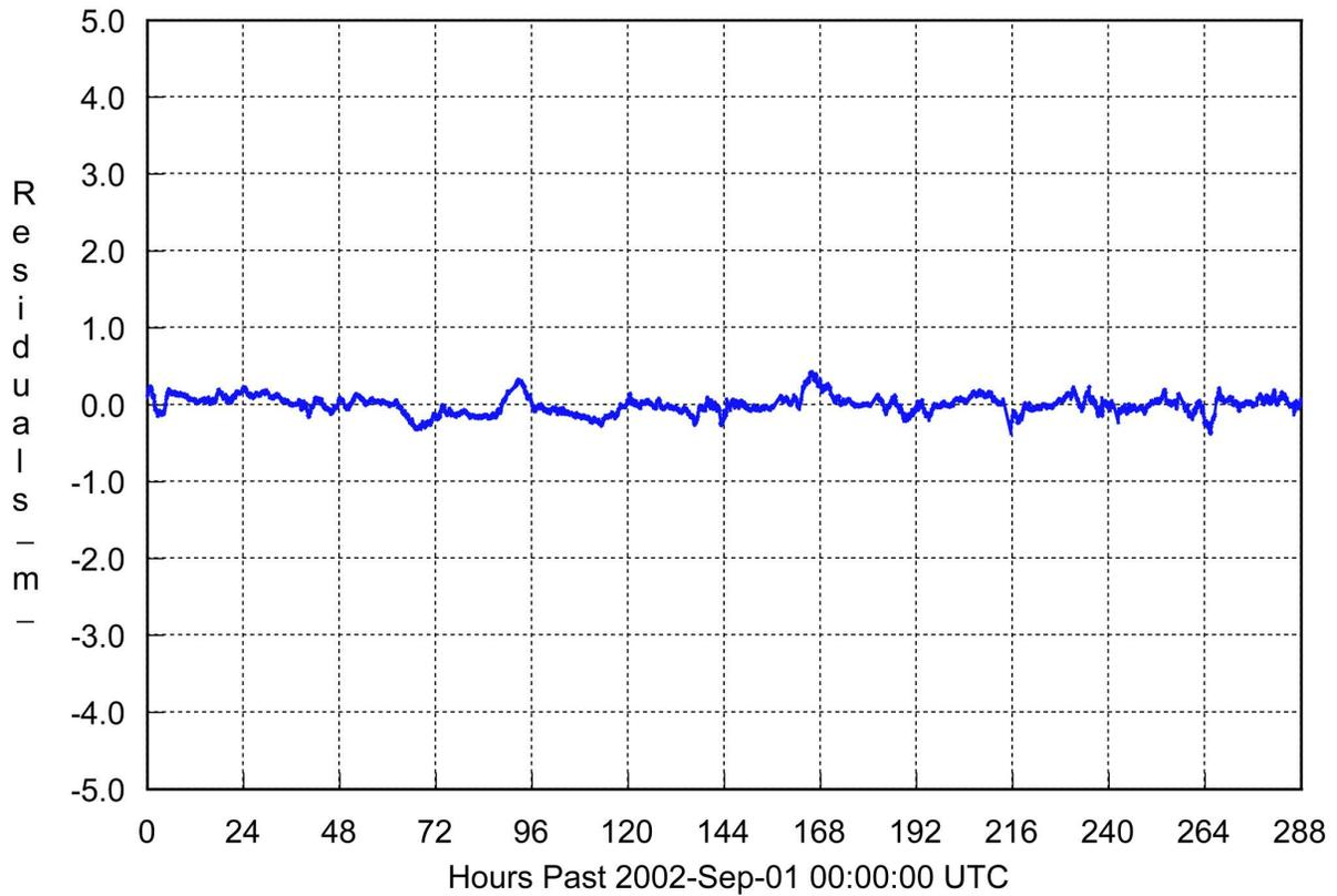
FIG.5 Post-Fit Geostationary Satellite Phase Residuals (10-Day Arc)
