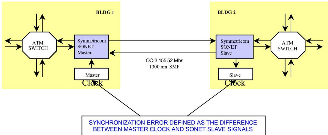
FIG.4 Typical Time-Based Communications Implementation
