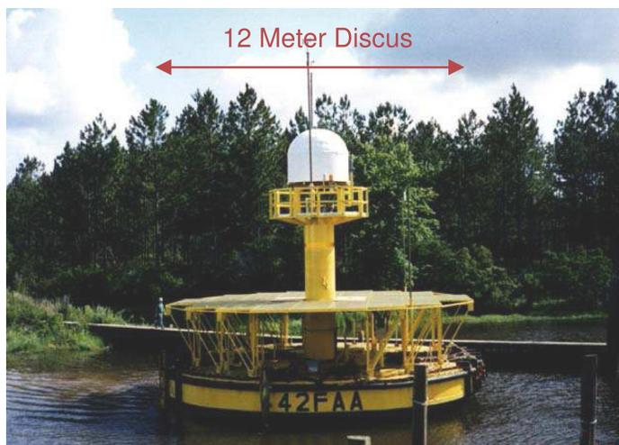
FIG. 11 Large Navigational "FAA" Buoy
