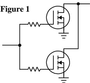
The most common method used to prevent the oscillation is to insert a resistor in series with each gate, typically 3 to 10 ohms, as shown in Figure 1. This is effective and economical but it reduces the HF gain of the pair.
