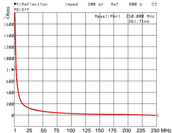
**Figure 10 Zener Impedance vs. Frequency, DO-41 Package**
