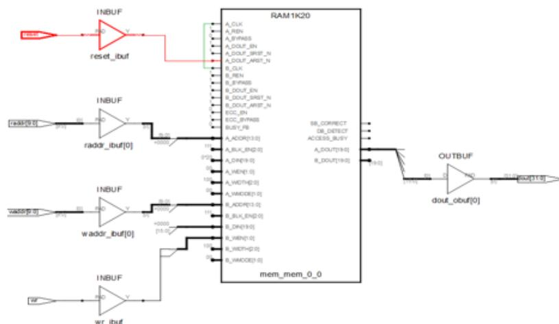
The tool infers PolarFire RAM1K20 with asynchronous reset packing.
