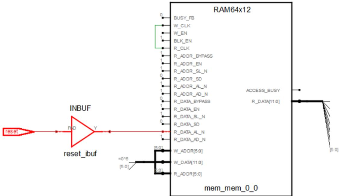
The tool infers PolarFire RAM64x12 with asynchronous reset packing.
