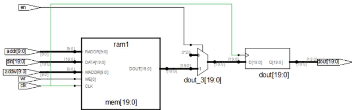
The tool infers one RAM1K20 using A\_BLK\_EN pin for enable en. enable en pin is mapped using A\_BLK\_EN or B\_BLK\_EN pin on LSRAM only when one port of RAM1K20 is used for reading and another port for writing.
