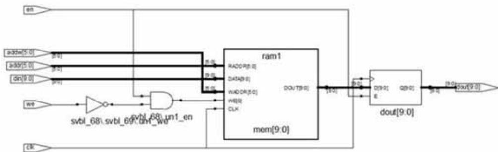
The tool infers PolarFire RAM64X12 with enable en packing.
