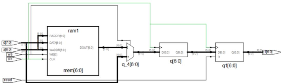
The tool infers PolarFire RAM64X12 with glue logic.
