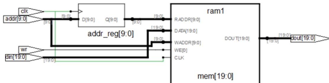
The synthesis tool infers PolarFire RAM1K20.
