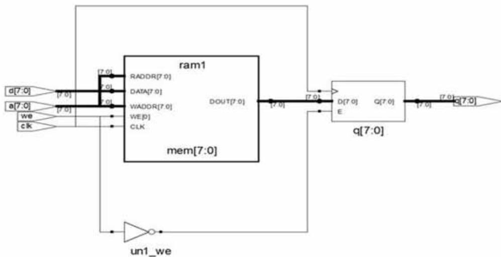
The tool infers PolarFire RAM1K20 along with logic for no change mode with enable en packing.
