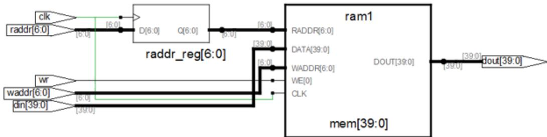
The FPGA synthesis tool infers PolarFire RAM1K20.
