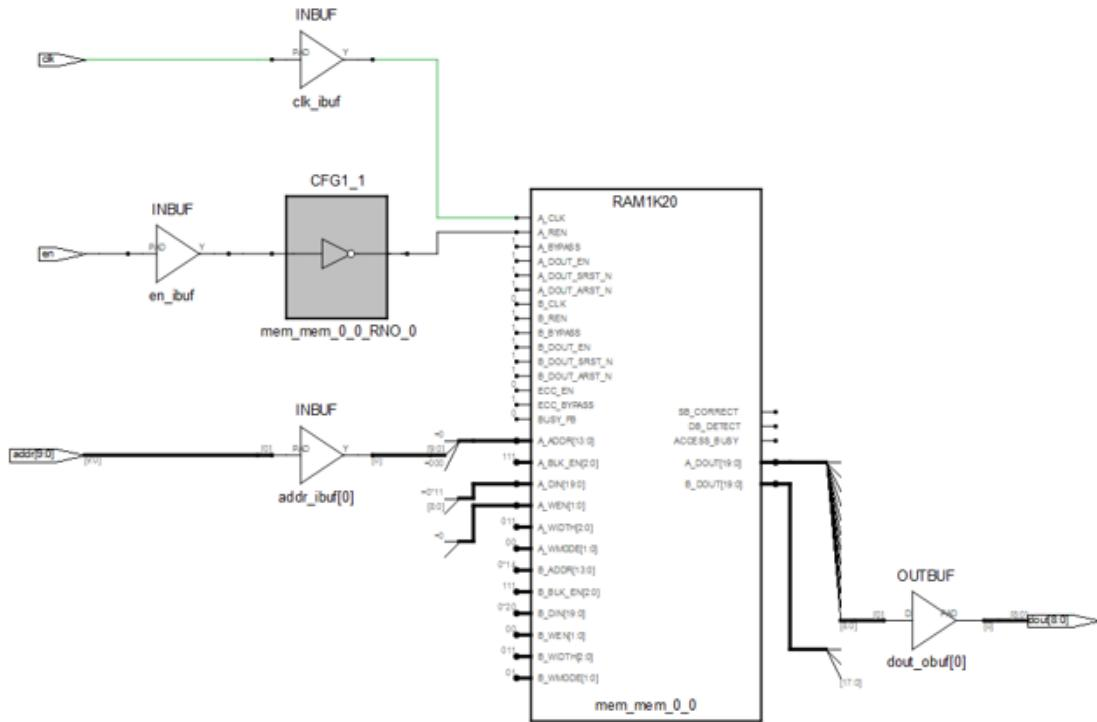
The tool infers PolarFire RAM1K20 without glue logic for read/write collision check with enable en packing.
