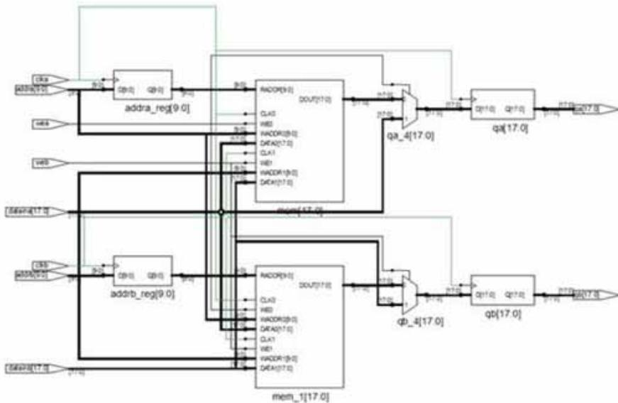
The tool infers PolarFire RAM1K20 with output registers qa and qb inferred outside the RAM using SLE's.
