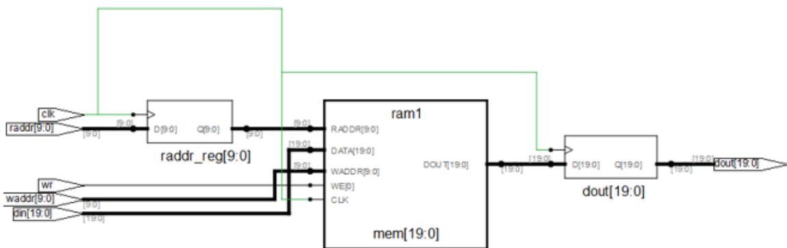
The FPGA synthesis tool infers PolarFire RAM1K20 along with glue logic for read/write address check.
